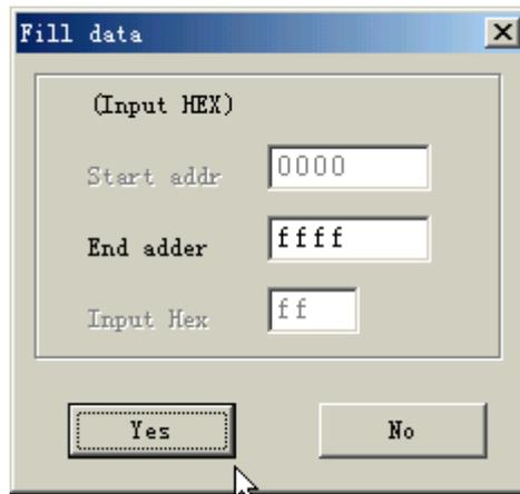
Data filling, extending or shrinking the file buffering zone can also be performed in the buffer zone area by clicking the right button of the mouse.
