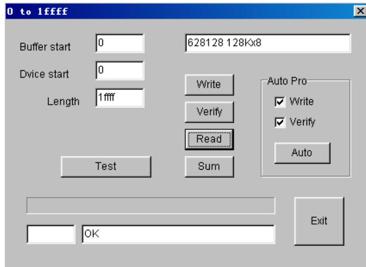
The menu is chiefly used to test the common static storage SRAM. Press Auto button, and the programmer tests each byte of memory to ensure the test is performed stably.
