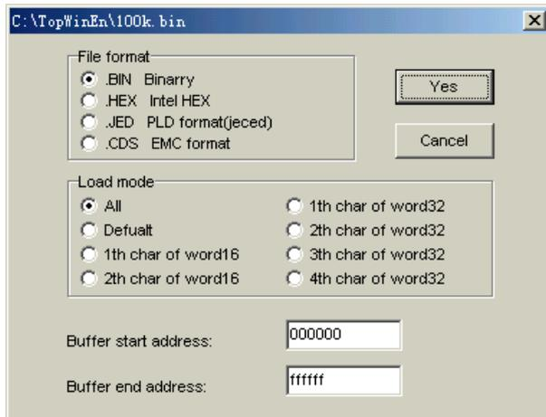
After confirming the file format, start and end address of buffer zone of the opening file, load the file data into the buffer zone, it will run as follow:
