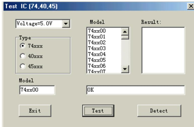
Select Series and Type of the tested device, and press testing button. In case that the device is normal, the speaker beeps a time, otherwise beeps three
