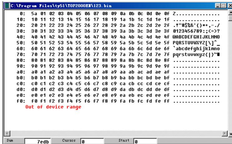
After the loading of file data into the buffer zone, if required to amend, move the mouse or keyboard to the relative byte and input the number directly. But the input number must be two hexadecimal numbers.
