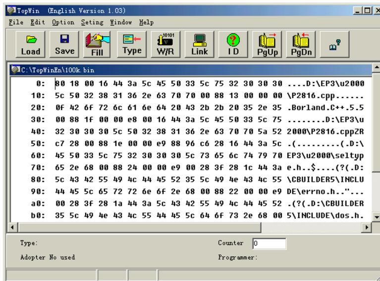
Software interface is composed by menu bar, toolbar, buffer zone, status bar and report group, therein five menus include all functions and options of TOPWin operation, set up common icon button in toolbar, it has the completely same effect to the operation which use in the menu. To use the methods of click can make command transfer more convenient and rapid.
