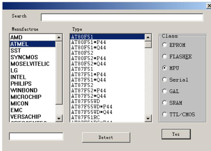
The procedures to select “Type” of device are to confirm the type of device in order of “Type->Manufacturer->Type”.
