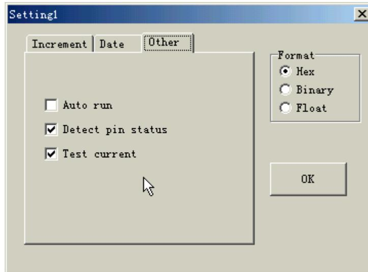
Quantity Mode: if allowable, press Auto button a time while writing a device, and then it can auto detect whether the device is pinned securely. Once the device is properly installed, the writing process starts instantly. After fully running a time, it will display "OK, Please take away the completed device". Once take away the device, it display "Place a new
