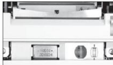
Cutter extending out and not at home position.
