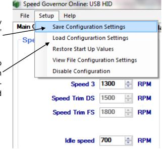
A particular and very helpful function is offered by the Start Up Values button. If you have adjusted the governor and cannot reproduce the original values (and have not stored these) this function can be used to retrieve them. The PC software saves the settings that were stored at the time the connected was established with the DDD100.
