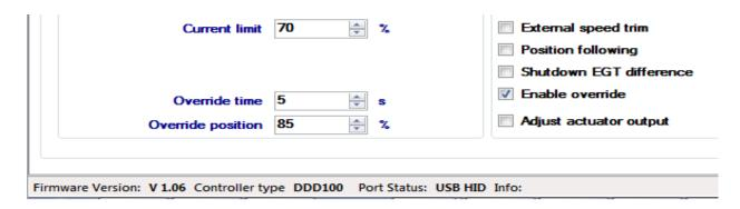
Override feature will start to work if the engine needed more fuel to compensate the sudden change in load of Genset in that case actuator opened up to override Position for set override time period after that come back to normal position within Current limit set value.
