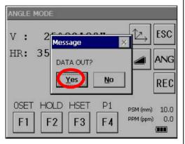
4 After the measurement, press the [Yes] key.
