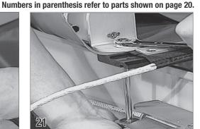
Secure the leading edge insert support bracket to the slider by placing the 10-32 X 1" screw up through the slider, the hole in the front corner of the cover, and through the support bracket. Tighten completely using 10-32 nylock, then back the nut off 1/2 turn.
