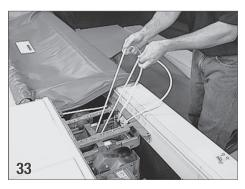
While holding the ropes over the mechanism, run the key switch in the cover position. The excess rope will be wrapped around the rope reel.
