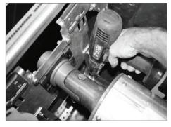
Anchor the mounting feet on both the motor and non motor ends of the mechanism in the houisng using as many anchor points as possible.
