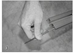
To determine the correct guide space for the cover system, measure the length of the roll up tube. The guide space should be three inches longer than the roll up tube length.
