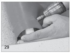
Position the fabric on the leading edge so it is in line with the leading edge support bracket. Secure with a tek screw on the back side of the leading edge. Be sure the screw does not interfere with the leading edge insert.
