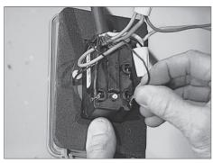
Attach the other leg from the indicator light and the **BLUE DIRECTIONAL WIRE** into terminal A1, and tighten the screw.
