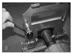
Install the feet on the non-motor end . The top of the pulley bracket should be flush with the top of the encapsulation.
