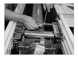
On the motor <u>and</u> non-motor side, use the half inch screws (27) and nylock nuts (29) provided and bolt the cross braces together.
