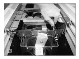
**Extending The Pulley Brackets**Loosen the nuts in the four positions on the adjustable brackets of the mechanism. Spread the brackets outward against the walls of the housing.
