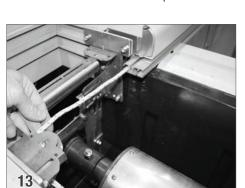
On the non motor end, make sure the rope will travel straight from the guide to the pulley.
