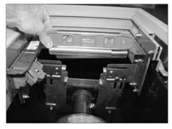
Now loosen the bolts and spread the pulley brackets at the non-motor end making sure they are also level. Anchor the bracket in as many points as possible.
