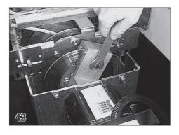
If further adjustment is needed, rotate the torque limiter brake arm to position the second brake bolt and tighten the second brake bolt 1/2 turn.
