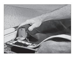
Pull the rope where it comes out of the guide as you feed the slider and cover into the guide a short distance.
