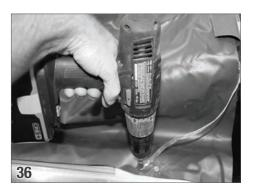
Lay the bond wire on top of the cover fabric. Secure it to the roll up tube using a tek screw (32). Distribute the slack of the cover evenly between each screw across the length of the tube. Secure the cover to the roll-up tube using tek screws (32) every 2-3ft. When attaching the cover to the tube, do not use folds or pleats.
