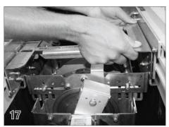
Raise the pulley brackets up so that the top of the bracket is even with the top of the encapsulation. This insures the ropes will be level.
