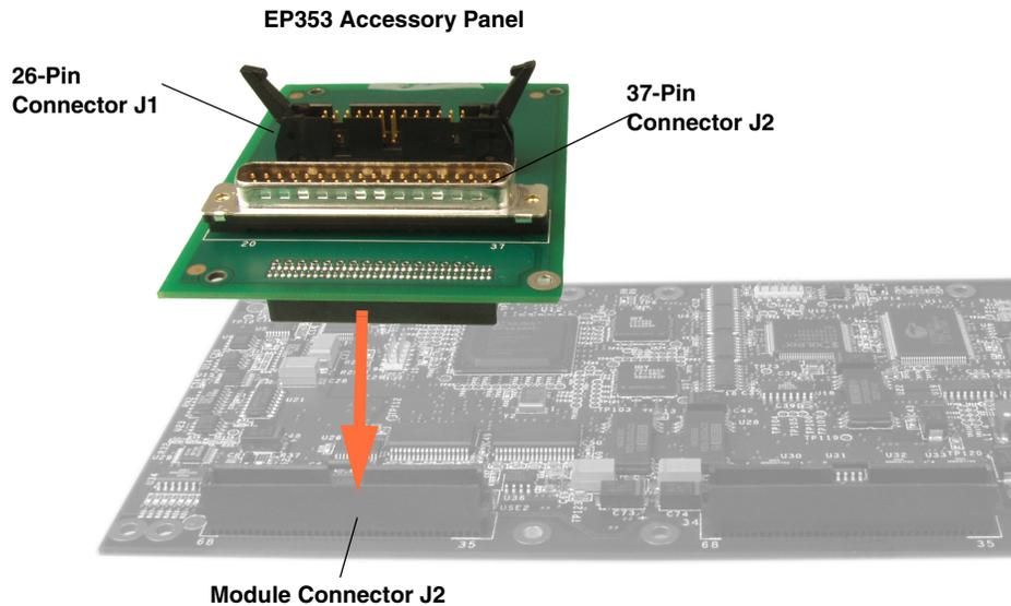
**Figure 33: Connecting the EP353 Accessory Panel to Connector J2 on the OEM Version of a DT9826 Series Module**
