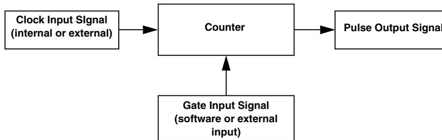
**Figure 24: Counter/Timer Channel**
