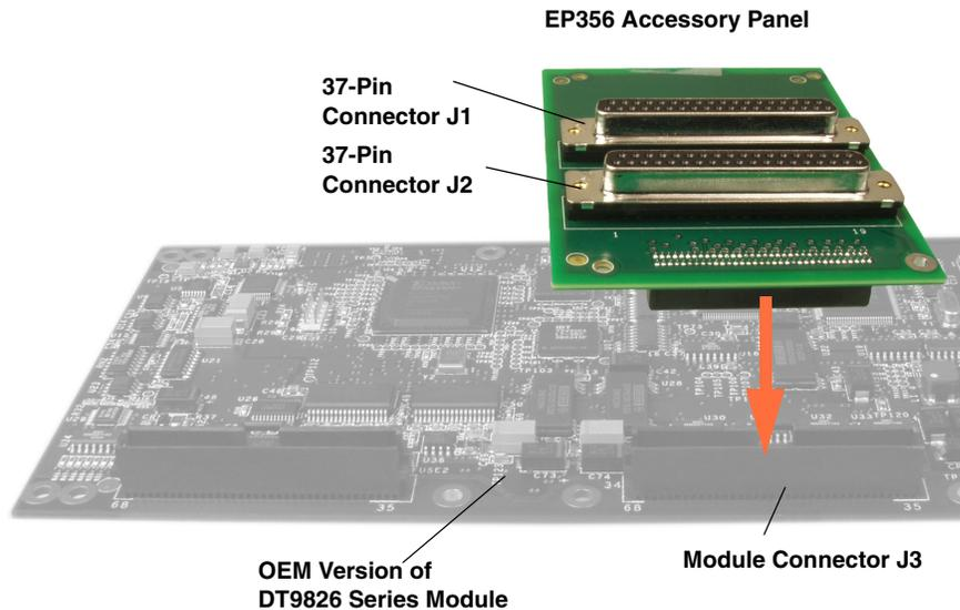
**Figure 38: Connecting the EP356 Panel to Connector J3 on the OEM Version of a DT9826 Series Module**
