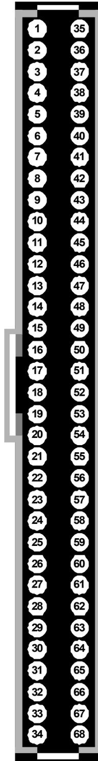
Figure 31: Layout of the 68-Pin Digital I/O Connector
