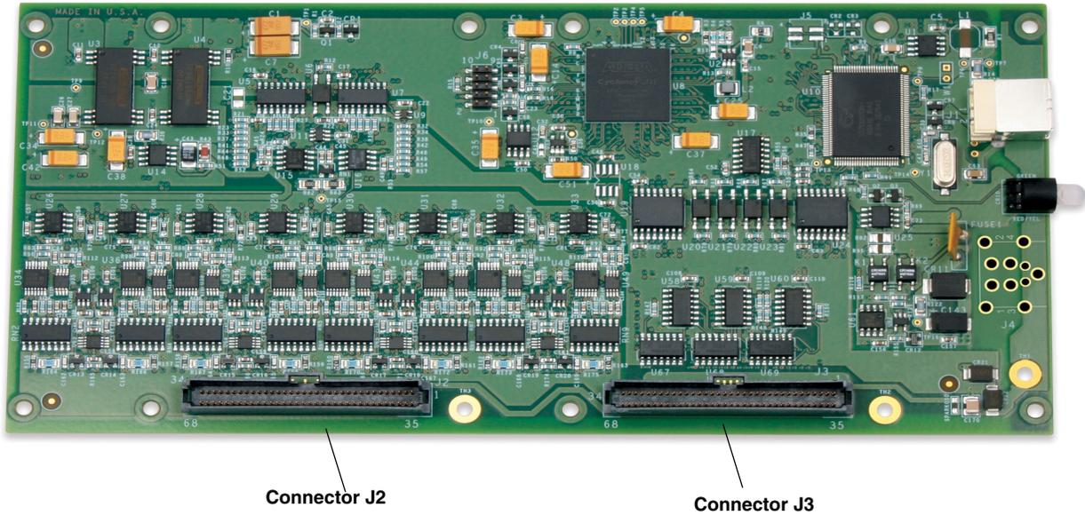
**Figure 32: Connectors on OEM Version of DT9826 Series Module**
