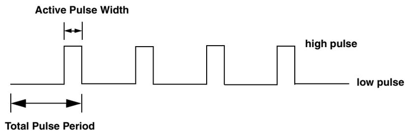
Figure 25: Example of a Low-to-High Pulse Output Type
