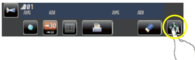
Auto : As soon as the alignment is OK, measurement is performed.
