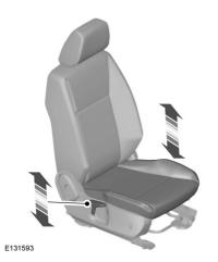
Each pull or press on the lever will raise or lower the height by a small amount.
