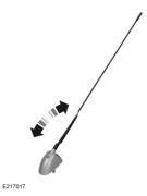
The radio aerial is mounted on the roof of the vehicle above the interior rear view mirror. It is can be raised and lowered. The aerial spire can be removed by unscrewing it from the base.
