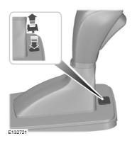
Use the button to move the selector lever from the park position in the event of an electrical malfunction or if your vehicle has a flat battery.
