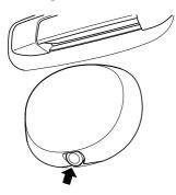
▼Switching the rear view camera on
