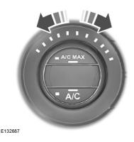
You can set the temperature between 16 °C (61 °F) and 28 °C (82 °F) in steps of 0.5 °C (1 °F). In position **LO** (below 16 °C (61 °F) the system will switch to permanent cooling, in **HI** (above 28 °C (82 °F) to permanent heating, and not regulate a stable temperature.
