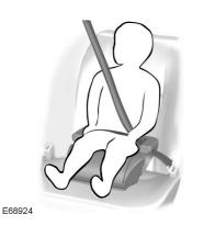
When using a booster cushion, always install the vehicle head restraint to the seat where the booster cushion is installed.
