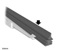
Run the tip of your fingers over the edge of the blade to check for roughness. Clean the wiper blade lips with water applied with a soft sponge.
