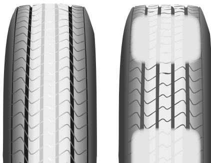
Figure 207: Centre Wear & Flat Spot Tyre Wear Patterns
