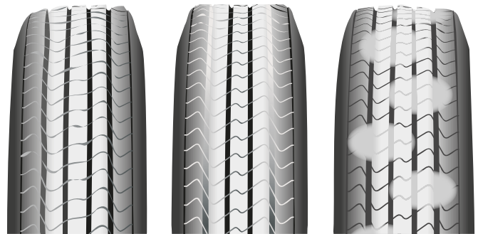
Figure 208: Feathered, Edge Wear, Cupped Wear Patterns
