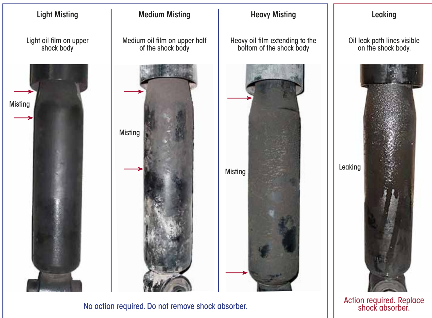
Figure 152: Shock Absorber Visual Inspection
