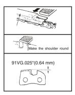
Be sure to round off the front edge of the depth gauge to reduce the chance of kickback or breakage. Make sure every link has the same length and edge angles as shown. Check using an appropriate gauge checker.
