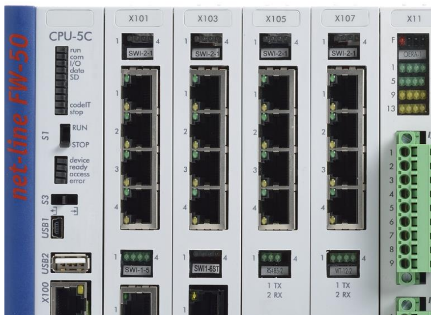
Figure 24: Example: Four SWI-2 at positions X101, X103, X105, X107
