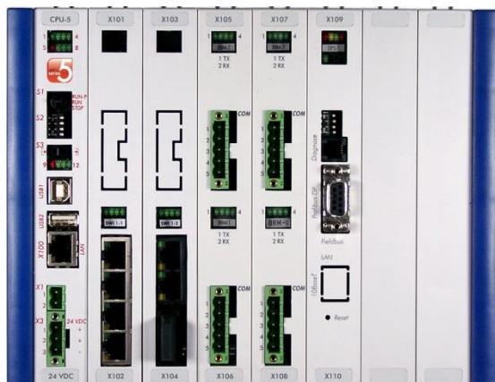
Figure 9: Example - net-line FW-50 with CPU-5 and pure router
