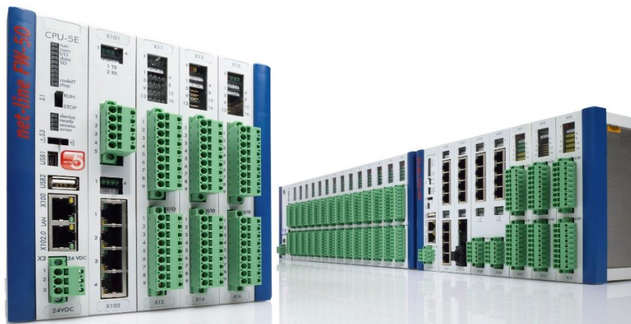
Figure 1: Product family FW-50 series5e, right FW-50 with 6 separated LAN segments
