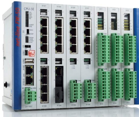
Figure 2: FW-50 series5e in BGT-M with 6 LAN segments, 2 serial interfaces and I/O cards
