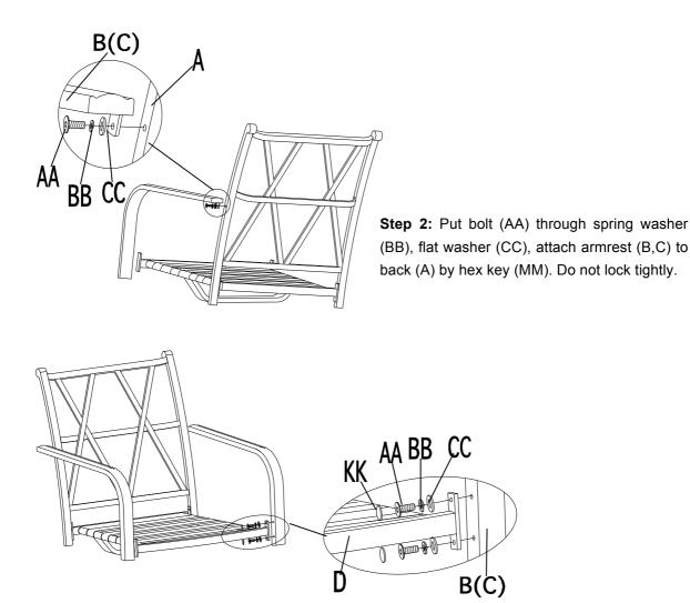
**Step 3:** Attach armrest (B,C) to seat (D) by bolt (AA), spring washer (BB), flat washer (CC) and hex key (MM). Put on cap (KK) after locking all bolts tightly.
