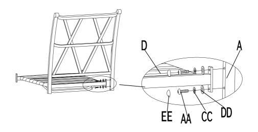
Step 1: Attach seat (D) to back (A) by bolt (AA), spring washer (BB), flat washer (CC) and hex key (MM). Do not lock tightly. Put on cap (KK) after locking all bolts tightly.
