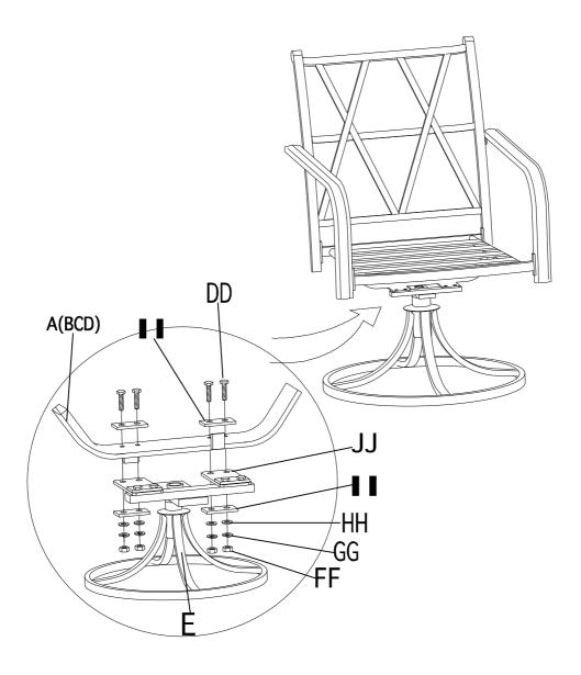
**Step 4:** Put hole of base (E) and hole of assembled frame A(BCD) on the same line, put screw (DD) through big washer (II), spring steel plate (JJ), big washer (II), flat washer (HH), spring washer (GG), attached nut (FF) by wrench (LL). Lock all bolts tightly by wrench (LL).
