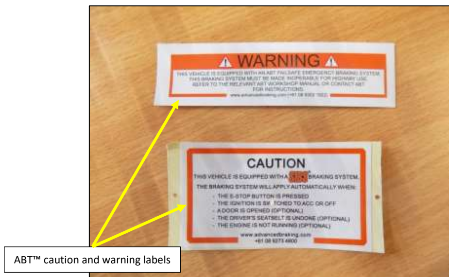
Figure 30: Failsafe Emergency labels.
