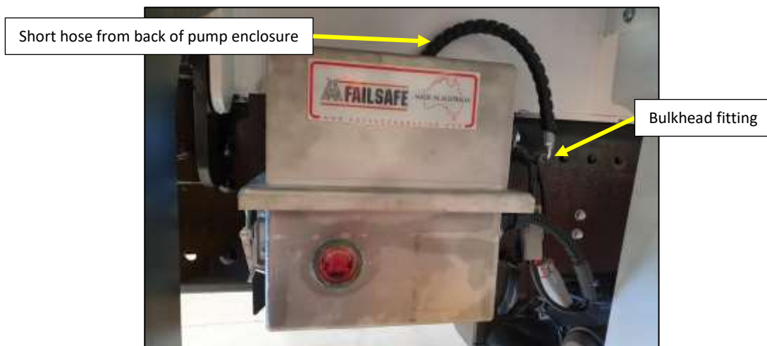
Figure 10: ABT™ Failsafe Emergency brake pump enclosure and hydraulic connections.
