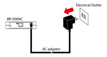
**2.** Press and hold the push switch on the front while inserting the AC adaptor back into the electrical outlet.
