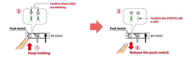
**6.** The BR-500AC and the Access Point will start to communicate each other. When the configuration finished successfully, the WLAN LED turns green and the STATUS LED turns or blinks green.
