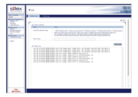
When the system log is saved, the event log and the other files are generated that will include the operating status.
