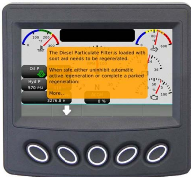
Figure 54 Orange Regen Caution Screen 1 Example of message that requires down soft key.
