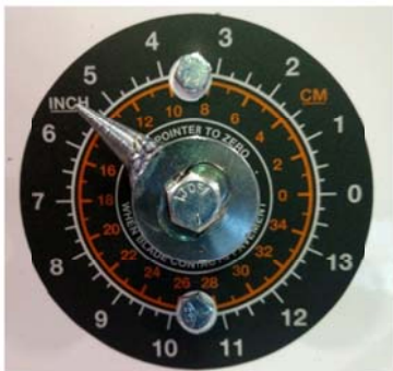
Figure 62: Cutting Depth Indicator
