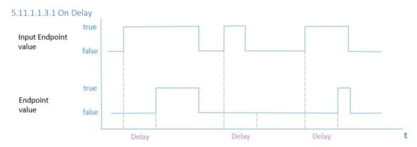
The value of the output *Endpoint* is set to true Delay [ms] time after a rising edge on the *Input Endpoint* has been detected. It is set to false as soon as a falling edge on the *Input Endpoint* has been detected. In case the period between a rising edge and a falling edge on the *Input Endpoint* is shorter than Delay [ms] time the value of the output *Endpoint* does not change.
