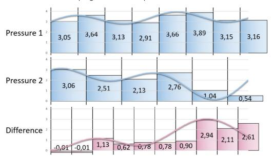
Result: The calculated difference differs (at the time of the calculation of the difference) compared with the real difference!
