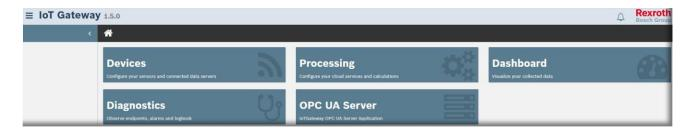
The modular structure allows adding and removing functionality on demand. Particular functions are displayed as tiles.
