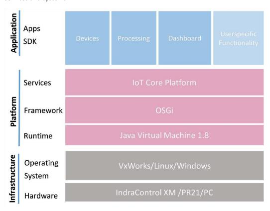
Running on the control system IndraControl XM there is a high performance combination of data acquisition with logic and motion processing in real time and large connectivity available. Via a SDK it is possible to create custom functions.
