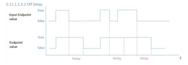
The value of the output *Endpoint* is set to true as soon as a rising edge has been detected on the *Input Endpoint*. It is set to false Delay [ms] time after a falling Edge has been detected on the *Input Endpoint*. In case the period between a falling edge and the following rising edge on the *Input Endpoint* is shorter than the configured Delay [ms] time the value of the output *Endpoint* does not change.
