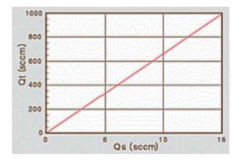
Bypass parts has applied a manufacturing technology that applied the patent technology to give the perfect alignment with guarantee. Flow measurements are done by the sensor, yet most of the flow flows by the bypass and is structured to have an alignment relationship where it can measure the entire flow.
