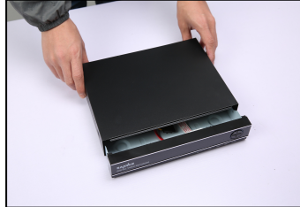
② disassemble the cover
