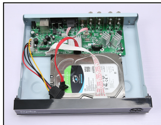
④ fix the screw of hard disk
