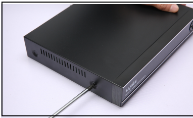
① disassemble the screw
