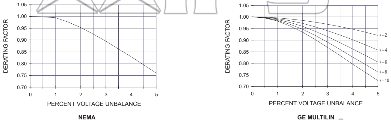
Figure 4-12: MEDIUM MOTOR DERATING FACTOR DUE TO UNBALANCED VOLTAGE
