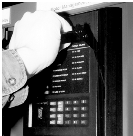
Figure 2-7: ROTATE HANDLE TO STOP POSITION
