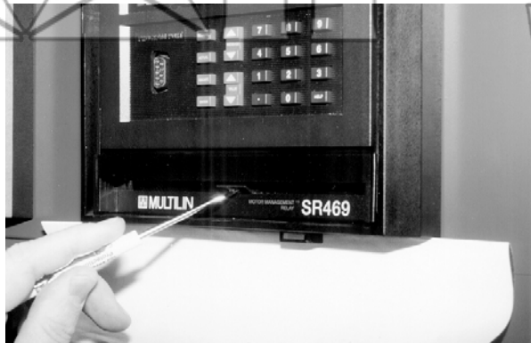
Figure 2-6: PRESS LATCH TO DISENGAGE HANDLE
