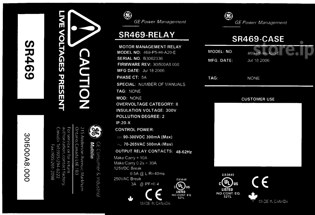
Figure 2-3: CASE AND UNIT IDENTIFICATION LABELS
