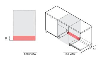
Service outlet at rear extends both sides, hoses and cords can be routed to either or both sides. Units shown in mm
