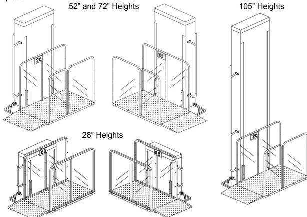
2/ The vertical side panels can be arranged for front exit from the platform.
