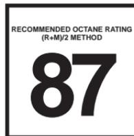
This engine is designed to meet all emissions regulations and provide excellent fuel economy and performance when using high-quality unleaded “Regular” gasoline having an octane
