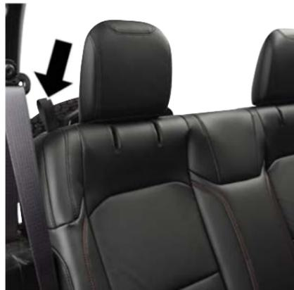
**Rear Head Restraint Folding Strap Location**
