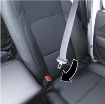
**Inserting Latch Plate Into Buckle**
