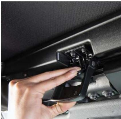
**Squeeze Latch Plate And Pull Handle Upward**
