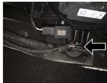
**Auxiliary Switch Connections – Under Instrument Panel**
