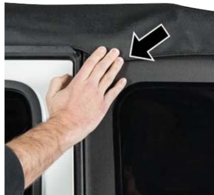
**Firmly Secure Hook-And-Loop Fastener**
