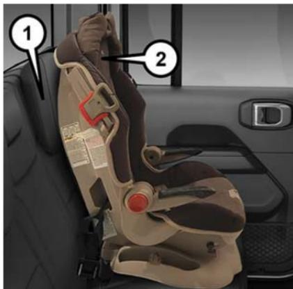
**Car Seat With Head Restraint Folded**
