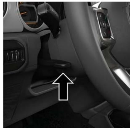
**Tilt/Telescoping Steering Column Lever**
