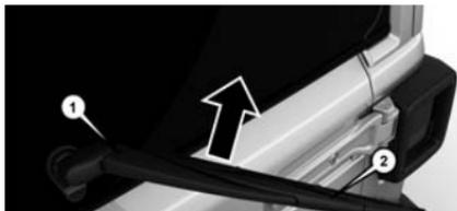
**Wiper Blade Removed From Wiper Arm**
