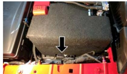
**Auxiliary Switch Connections – Under Hood**
