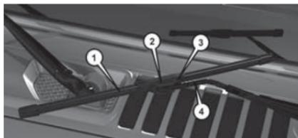
**Wiper Blade With Release Tab In Locked Position**
