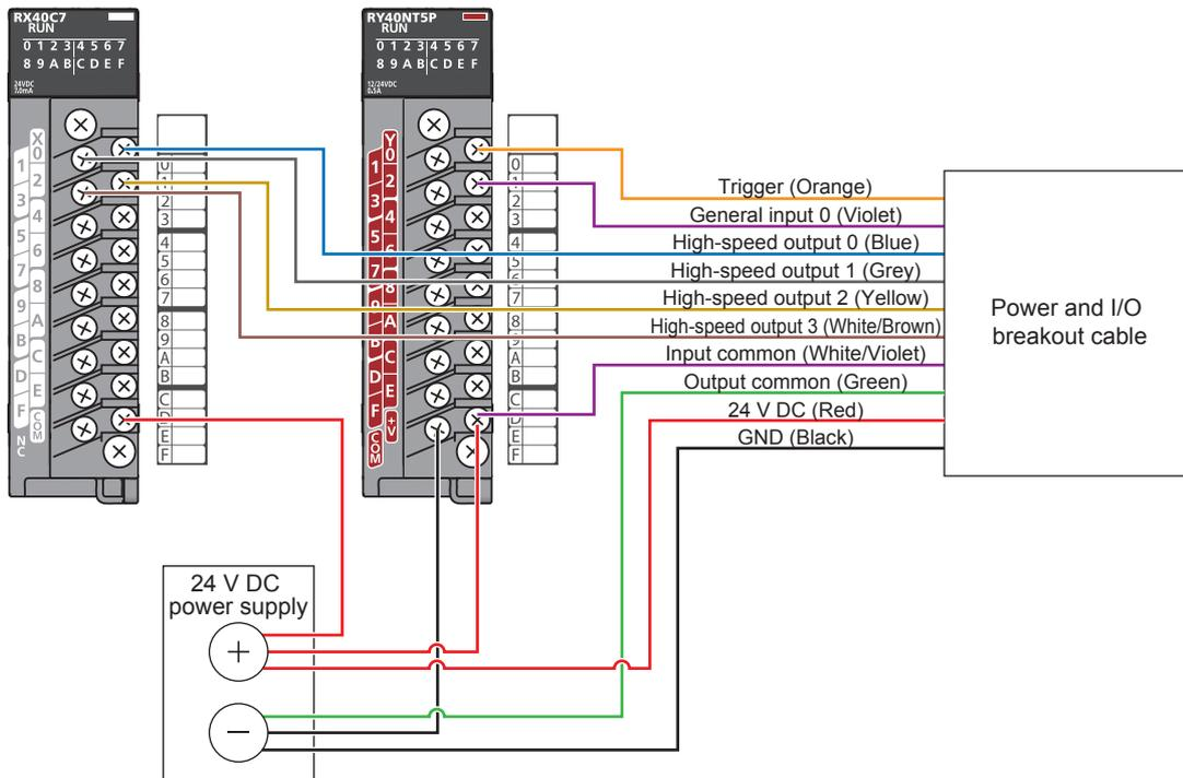
3. Connect the power and I/O breakout cable's M12 connector to the vision sensor's Power, I/O and RS-232 connector.
