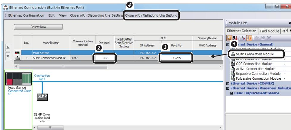
① Select "SLMP Connection Module" from the module list and paste by drag&drop.
