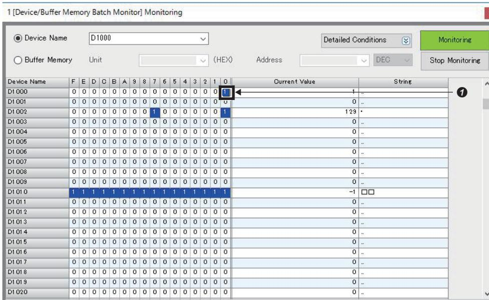
① To enable the trigger from the programmable controller, turn "ON" the "Network Trigger Enable" bit (D1000.0) of the control bit block. When the "Network Trigger Enable" bit (D1000.0) is "OFF", the vision sensor does not operate even though the trigger is ON.
