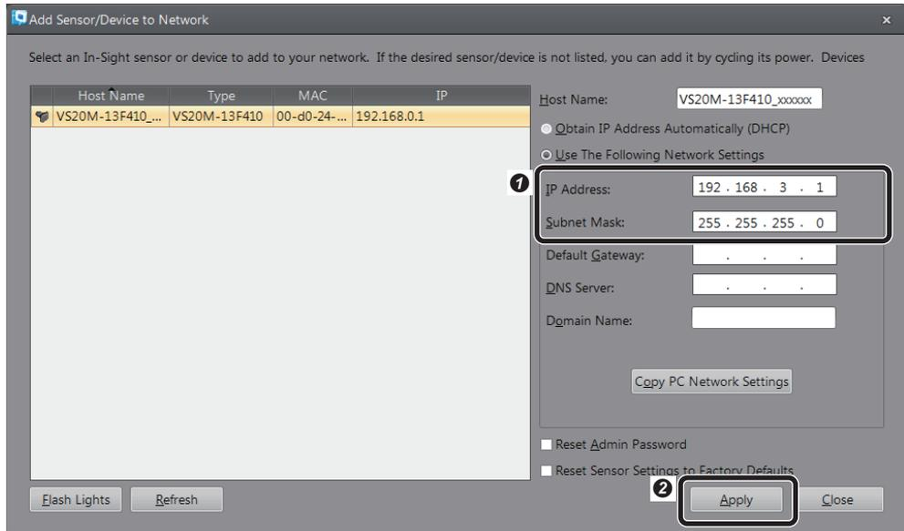
1 Add the sensor and device to the network as shown left.
