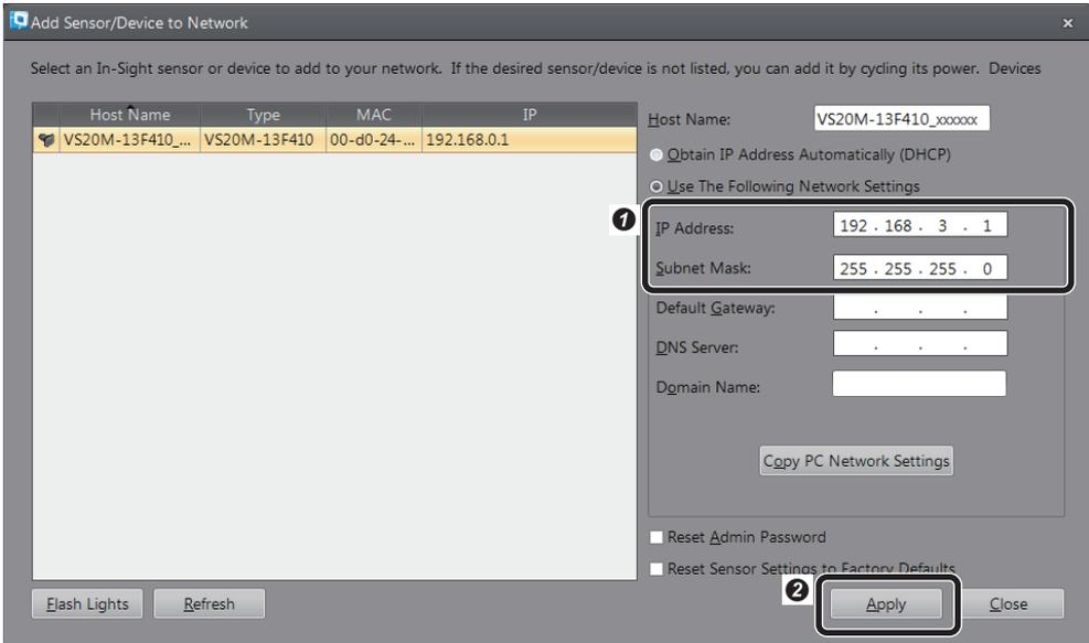
1 Set the sensor and device to the network as shown left.
