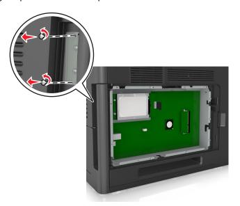
4 Remove the printer hard disk.
