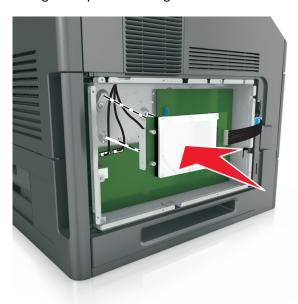
**Note:** Make sure the cables are neatly tucked under the printer hard disk.
