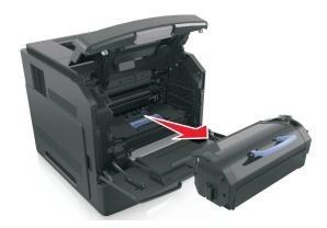
**3** Lift the blue handle, and then pull out the imaging unit from the printer.
