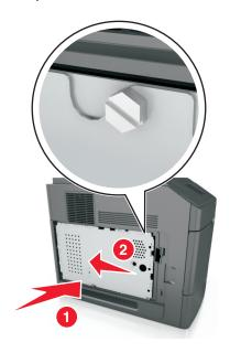
**6** Tighten the screws on the shield.
