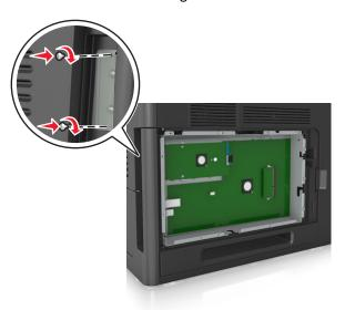
**10** Tighten the thumbscrew that is attached to the ISP.
