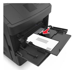
**Warning—Potential Damage:** Never use envelopes with stamps, clasps, snaps, windows, coated linings, or self-stick adhesives. These envelopes may severely damage the printer.
