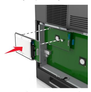
**c** Insert the plug of the printer hard disk interface cable into the receptacle of the ISP.
