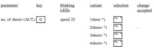
\*) Since the ECG memory accepts a maximum of 10 seconds, it is recommended to select only 1 or 2 sheets for a recording speed of 25 mm/s, or 1 sheet for 5 mm/s.
