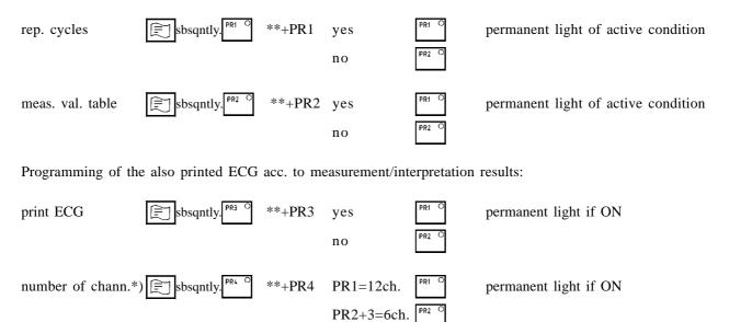
\*) ECG recording using the PR1 (12 channels), or successively using PR2 and PR3. \*\*) blinking LEDs: speed, sensitivity
