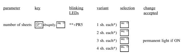
\*) Since the ECG memory can store max. 10 seconds, it is advisable to select only 1 or 2 sheets for recording at 25 mm/sec, and only 1 sheet for 5 mm/sec.
