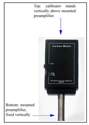
FIGURE 2-1 Vertical Positioning
