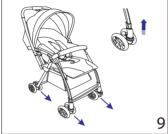
Unlocking and rotating the front wheels and rear wheels. Push downward the positioning lock of the front wheel and rear wheel until hearing a "click" sound. The front wheel and rear wheel are unlocked and can be rotated.
