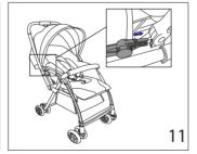
Activating the brake. To activate brake: Push the brake arm downward with your foot until hearing a "click". To release brake: Pull the brake arm upward with your foot.
