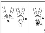
Assembling the front bumper. Insert the front bumper to the opening position of the stroller frame along the direction of the arrow as shown until it locks up in place.
