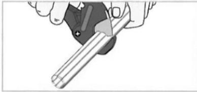
Cut the tube square and remove burrs and sharp edges. Ensure the outside diameter is free of score marks. For soft or thin walled tube we recommend the use of a tube insert
