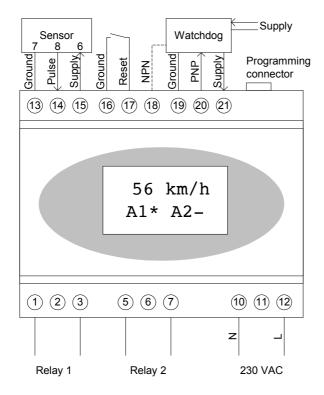
Power supply 230 V is brought to connectors 10 and 12. Ground connection is not needed.
