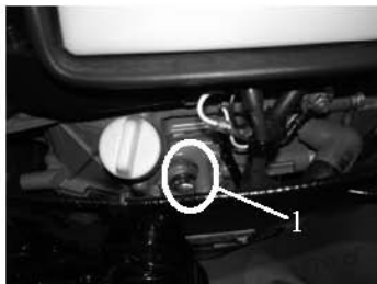
1.oil level check window
