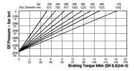
Maximum Braking Force SH 8.4: 19.5kN (4383.77 lbf) Minimum Pressure for full retraction: 65 bar (943 psi) Weight of caliper and thruster - 50.2kg (110.67 lb) Weight of thruster only - 16.2kg (35.71 lb)
