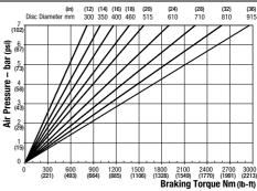
Maximum Pressure 7 bar (102 psi) Maximum Braking Force = 6.9kN @ 7 bar (1551.18 lbf @ 102 psi) Weight of caliper and thruster - 8.32kg (18.39 lb)
