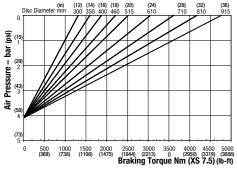
Minimum Pressure for full retraction: 5.5 bar (80 psi) Maximum Braking Force XS 7.5: 11.2kN (517.86 lbf) Weight of caliper and thruster - 11.9kg (26.23 lb) Weight of thruster only - 4.9kg (10.80 lb) Volume displacement of thruster at full retraction = 1.19ml (0.06 fl oz)
