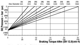
Maximum Braking Force SH 12.9: 30kN (6744.27 lbf) Minimum Pressure for full retraction: 100 bar (1450 psi) Weight of caliper and thruster - 52kg (114.64 lb) Weight of thruster only - 18kg (39.68 lb) Volume displacement of thruster at full retraction = 56ml (1.89 fl oz)
