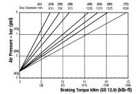
Maximum Braking Force SD 12.9: 30kN (6744.27 lbf) Minimum Pressure for full retraction: 3.8 bar (55 psi) Weight of caliper and thruster - 54kg (119.05 lb) Weight of thruster only - 20kg (44.09 lb) Volume displacement of thruster at full retraction = 2.51ml (0.08 fl oz)
