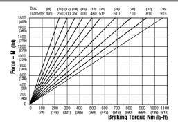
Weight of MR caliper and hand wheel assembly - 7.8kg (17.19 lb) Weight of MR2 caliper and hand wheel -8.3kg (18.29 lb) Weight of hand wheel assembly only - 1.3kg (2.86 lb) Maximum Braking Force = 2.68kN (602.48 lbf)
