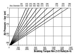
Minimum Pressure for full retraction: 2.5 bar (36 psi) Maximum Braking Force 1/2 rate: 3.2kN (719.38 lbf) Weight of caliper and thruster - 10.5kg (23.14 lb) Weight of thruster only - 3.5kg (7.71 lb) Volume displacement of thruster at full retraction = 950ml (32.12 fl oz)
