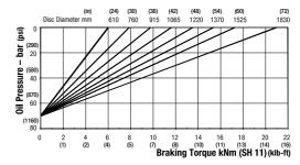
Maximum Braking Force SH 11: 25kN (5620.22 lbf) Minimum Pressure for full retraction: 92 bar (1334 psi) Weight of caliper and thruster - 51.2kg (112.88 lb) Weight of thruster only - 17.2kg (37.92 lb) Volume displacement of thruster at full retraction = 56ml (1.89 fl oz)
