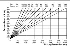
Weight of MR caliper and thruster - 7.9kg (17.41 lb) Weight of MR2 caliper and thruster - 8.4kg (18.51 lb) Weight of lever assembly only - 1.4kg (3.08 lb) Maximum Braking Force = 8.3kN @ 0.9kN 1865.91 @ 202.33 lbf) force on lever
