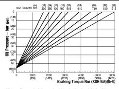
Minimum Pressure for full retraction: 82 bar (1189 psi) Maximum Braking Force XSH 9.6: 14.3kN (3214.76 lbf) Weight of caliper and thruster - 11.6kg (25.57 lb) Weight of thruster only - 4.6kg (10.14 lb) Volume displacement of thruster at 6mm (0.24 in) retraction = 9.1ml (0.30 fl oz)
