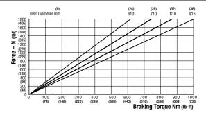
Weight of caliper and hand wheel assembly - 10.52kg (23.19 lb) Weight of hand wheel assembly only - 1.3kg (2.87lb) Maximum Braking Force = 2.68kN (602.49 lbf)
