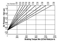
Minimum Pressure for full retraction: 33 bar (479 psi) Maximum Braking Force 2/3 rate: 4.3kN (966.67 lbf) Weight of caliper and thruster - 11kg (24.25 lb) Weight of thruster only - 4.0kg (8.81 lb) Volume displacement of thruster at 4mm (0.16 in) retraction = 5ml (0.16 fl oz)
