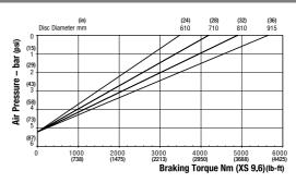
Maximum Braking Force XS 9.6: 14.3kN (3214.77 lbf) Minimum Pressure for full retraction: 6.5 bar (94 psi) Weight of caliper and thruster - 14.32kg (31.57 lb) Weight of thruster only - 5.1kg (11.24 lb) Volume displacement of thruster at full retraction = 1.19ml (0.06 fl oz)
