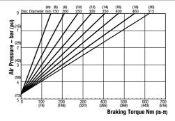
Maximum Pressure = 7 bar (102 psi) Minimum Pressure for full retraction = 6.2 bar (89.92 psi) Maximum Braking Force = 2.6kN (584.50 lbf) Weight of caliper and thruster – 2.24kg (4.94 lb) Weight of thruster only – 1.49kg (3.28 lb) Volume displacement of thruster at full retraction = 46ml (1.56 fl oz)
