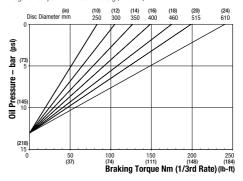
Maximum Braking Force 1/3rd rate: 0.87kN
