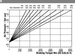
Minimum Pressure for full retraction: 6.4 bar (93 psi) Maximum Braking Force XS 9.6: 14.3kN (3214.76 lbf) Weight of caliper and thruster - 12.1kg (26.67 lb) Weight of thruster only - 5.1kg (11.24 lb) Volume displacement of thruster at full retraction = 1.19ml (0.06 fl oz)
