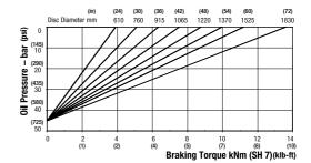
Maximum Braking Force SH 7: 16.5kN (3709.35 lbf) Minimum Pressure for full retraction: 59 bar (856 psi) Weight of caliper and thruster - 49.7kg (109.57 lb) Weight of thruster only - 15.7kg (34.61 lb) Volume displacement of thruster at full retraction = 56ml (1.89 fl oz)
