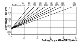
Maximum Braking Force SH 2.5: 6kN (1348.85 lbf) Minimum Pressure for full retraction: 21 bar (305 psi) Weight of caliper and thruster - 47.9kg (105.60 lb) Weight of thruster only - 13.9kg (30.64 lb) Volume displacement of thruster at full retraction = 56ml (1.89 fl oz)
