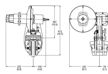
Maximum Braking Force = 6kN (1348.85 lbf) Weight of caliper and actuator - 17.9kg (39.46 lb)
