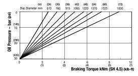
Maximum Braking Force SH 4.5: 10.5kN (2360.49 lbf) Minimum Pressure for full retraction: 38 bar (551 psi) Weight of caliper and thruster - 48.7kg (107.37 lb) Weight of thruster only - 14.7kg (32.41 lb) Volume displacement of thruster at full retraction = 56ml (1.89 fl oz)
