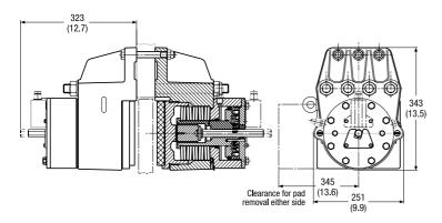
The Twiflex VKSD disc brake caliper is comprised of two halves, or spring modules, and is suitable for use with a minimum disc thickness of 20mm (0.79 in). The modules are mounted each side of a central mounting plate 12mm (0.47 in) thicker than the brake disc. Minimum disc diameter is 1000mm (39.37 in).
