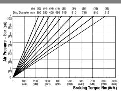
Maximum Pressure 7 bar (102 psi) Maximum Braking Force = 1.9kN @ 7 bar (427.13 lbf @ 102 psi) Weight of caliper and thruster - 7.3kg (16.09 lb)
