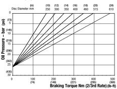
Maximum Braking Force 2/3rd rate: 1.74kN (391.17lbf) Minimum Pressure for full retraction: 33 bar (479 psi) Weight of caliper and thruster - 5.5kg (12.13 lb)
