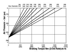
Minimum Pressure for full retraction: 3.3 bar (48 psi) Maximum Braking Force 2/3 rate: 4.3kN (966.67 lbf) Weight of caliper and thruster - 10.5kg (23.14 lb) Weight of thruster only - 3.5kg (7.71 lb) Volume displacement of thruster at full retraction = 950ml (32.12 fl oz)
