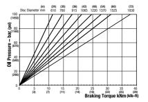
Maximum Pressure 100 bar (1450 psi) Maximum Braking Force = 45kN @ 100 bar (10116.40 lbf @ 1450 psi) Weight of caliper - 18.6kg (41.08 lb)
