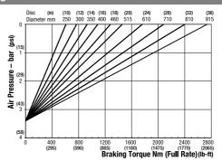
Minimum Pressure for full retraction: 5 bar (73 psi) Maximum Braking Force full rate: 6.4kN (1438.77 lbf) Weight of MR caliper and thruster - 10.0kg (22.04 lb) Weight of MR2 caliper and thruster - 10.5kg (23.14 lbf) Weight of thruster only - 3.5kg (7.71 lb) Volume displacement of thruster at full retraction is 950ml (32.12 fl oz)
