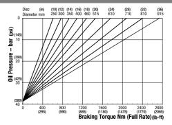
Minimum Pressure for full retraction: 50 bar (725 psi) Maximum Braking Force full rate: 6.4kN (1438.17 lbf) Weight of MR caliper and thruster - 10.5kg (23.14 lb) Weight of MR2 caliper and thruster - 11kg (24.25 lb) Weight of thruster only - 4kg (8.81 lb) Volume displacement of thruster at 4mm (0.16 in) retraction = 5ml (0.16 fl oz)
