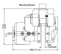
The Twiflex VCS-FL disc brake caliper comprises a single spring module forming the 'active' side of this floating unit and is available for use where space is limited or to accommodate axial disc float of ±6mm (0.24 in).
