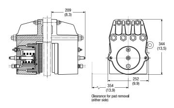
The Twiflex VKHD disc brake caliper is comprised of two halves, or hydraulic modules, and is suitable for use with a minimum disc thickness of 20mm (0.79 in). The modules are mounted each side of a central mounting plate 12mm (0.47 in) thicker than the brake disc. Minimum disc diameter is 1000mm (39.37 in).
