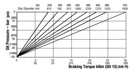
Maximum Braking Force SH 15: 35kN (868.31 lbf) Minimum Pressure for full retraction: 120 bar (1740 psi) Weight of caliper and thruster - 53kg (116.84 lb) Weight of thruster only - 19kg (41.89 lb) Volume displacement of thruster at full retraction = 56ml (1.89 fl oz)
