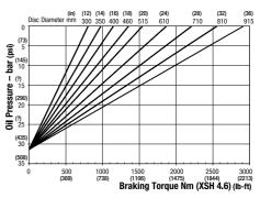
Minimum Pressure for full retraction: 40 bar (580 psi) Maximum Braking Force XSH 4.6: 6.8kN (1528.70 lbf) Weight of caliper and thruster - 11kg (24.25 lb) Weight of thruster only - 4kg (8.81 lb) Volume displacement of thruster at 6mm (0.24 in) retraction = 9.1ml (0.30 fl oz)
