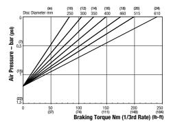
Maximum Braking Force 1/3rd rate: 0.87kN (195.58 lbf) Minimum Pressure for full retraction: 1.7 bar (25 psi) Weight of caliper and thruster - 4.9kg (10.80 lb)
