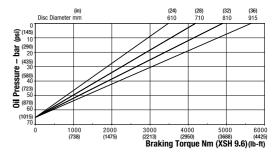
Maximum Braking Force XSH 9.6: 14.3kN (3214.77 lbf) Minimum Pressure for full retraction: 82 bar (1189 psi) Weight of caliper and thruster - 13.82kg (30.47 lb) Weight of thruster only - 4.6kg (10.14 lb) Volume displacement of thruster at 6mm (0.24 in) retraction = 9.1ml (0.30 fl oz)
