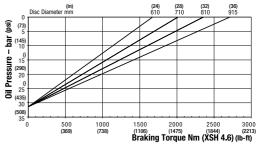
Maximum Braking Force XSH 4.6: 6.8kN (1528.70 lbf) Minimum Pressure for full retraction: 40 bar (580 psi) Weight of caliper and thruster - 13.22kg (29.15 lb) Weight of thruster only - 4kg (8.82 lb) Volume displacement of thruster at 6mm (0.24 in) retraction = 9.1ml (0.30 fl oz)
