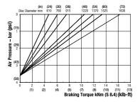
Maximum Braking Force S 8.4: 19.5kN (4383.77 lbf) Minimum Pressure for full retraction: 4.8 bar (70 psi) Weight of caliper and thruster - 46.2kg (101.85 lb) Weight of thruster only - 12.2kg (26.89 lb) Volume displacement of thruster at full retraction = 1.31ml (0.04 fl oz)
