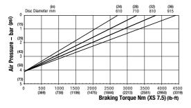
Maximum Braking Force XS 7.5: 11.2kN (2517.86 lbf) Minimum Pressure for full retraction: 5 bar (73 psi) Weight of caliper and thruster - 14.12kg (31.13 lb) Weight of thruster only - 4.9kg (10.80 lb) Volume displacement of thruster at full retraction = 1.19ml (0.06 fl oz)
