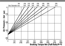
Maximum Braking Force full rate: 2.6kN (584.50 lbf) Minimum Pressure for full retraction: 5 bar (73 psi) Weight of caliper and thruster - 4.9kg (10.80 lb)
