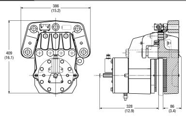
The Twiflex VKSD-FL disc brake caliper comprises a single spring module forming the 'active' side of this floating unit and is available for use where space is limited or to accommodate axial disc float of ±6mm (0.24 in).
