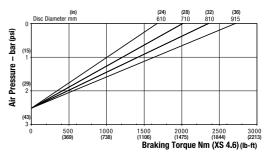
Maximum Braking Force XS 4.6: 6.8kN (1528.70 lbf) Minimum Pressure for full retraction: 3 bar (44 psi) Weight of caliper and thruster - 13.72kg (30.25 lb) Weight of thruster only - 4.5kg (9.92 lb) Volume displacement of thruster at full retraction = 1.19ml (0.06 fl oz)
