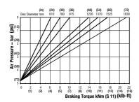
Maximum Braking Force S 11: 25kN (5620.22 ibf) Minimum Pressure for full retraction: 6 bar (87 psi) Weight of caliper and thruster - 47.2kg (104.06 lb) Weight of thruster only - 13.2kg (29.10 lb) Volume displacement of thruster at full retraction = 1.31ml (0.04 fl oz)
