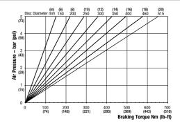
Maximum Pressure 5 bar (73 psi) Maximum Braking Force = 2.75kN@ 5 bar (618.22 lbf @ 73 psi) Weight of caliper and thruster - 1.9kg (4.19 lb) Weight of thruster only - 1.15kg (2.54 lb) Volume displacement of thruster at 13mm stroke = 46ml (1.56 fl oz)
