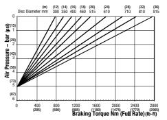
Minimum Pressure for full retraction: 5 bar (73 psi) Maximum Braking Force full rate: 6.4kN (1438.77 lbf) Weight of caliper and thruster - 10.5kg (23.14 lb) Weight of thruster only - 3.5kg (7.71 lb) Volume displacement of thruster at full retraction = 950ml (32.12 oz)
