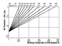
Minimum Pressure for full retraction: 1.7 bar (25 psi) Maximum Braking Force 1/3rd rate: 2.2kN (494.57 lbf) Weight of MR caliper and thruster - 10.0kg (22.24 lb) Weight of MR2 caliper and thruster - 10.5kg (23.14 lbf) Weight of thruster only - 3.5kg (7.71 lb) Volume displacement of thruster at full retraction is 950ml (32.12 fl oz)
