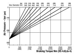
Minimum Pressure for full retraction: 3.1 bar (45 psi) Maximum Braking Force XS 4.6: 6.8kN (528.70 lbf) Weight of caliper and thruster - 11.5kg (25.35 lb) Weight of thruster only - 4.5kg (9.92 lb) Volume displacement of thruster at full retraction = 1.19ml (0.06 fl oz)
