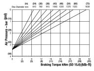
Maximum Braking Force SD 15.6: 36kN (8093.12 lbf) Minimum Pressure for full retraction: 4.6 bar (67 psi) Weight of caliper and thruster - 55kg (121.25 lb) Weight of thruster only - 21kg (46.29 lb) Volume displacement of thruster at full retraction = 2.51ml (0.08 fl oz)
