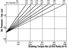
Maximum Braking Force 2/3rd rate: 1.74kN (391.17 lbf) Minimum Pressure for full retraction: 3.3 bar (48 psi) Weight of caliper and thruster - 4.9kg (10.80 lb)
