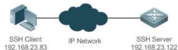
Figure 9-4 Network Topology for Public Key Authentication of SSH Users
