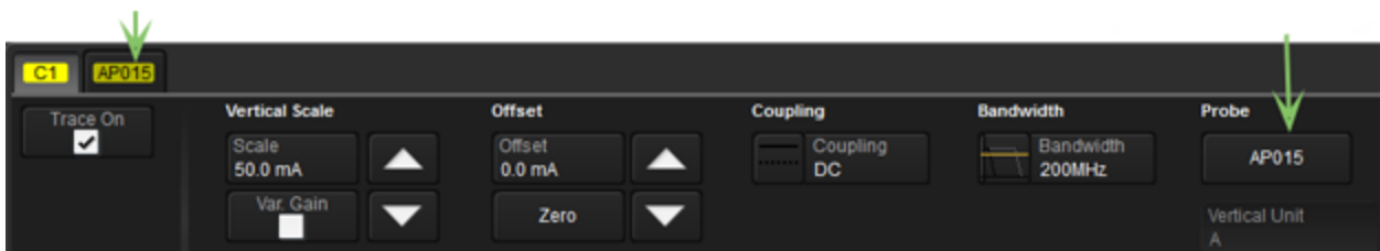
Channel dialog with tab for connected probe.
