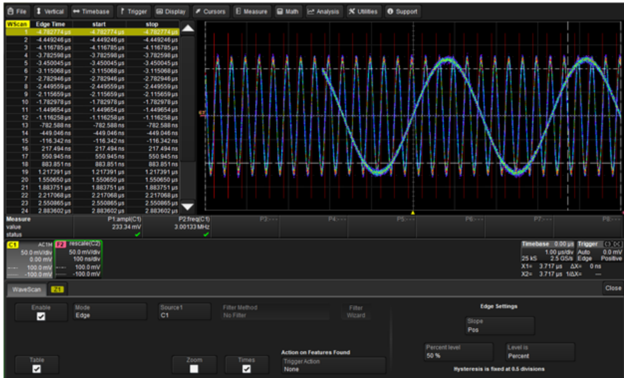
WaveScan window with all scan "views" turned on.
