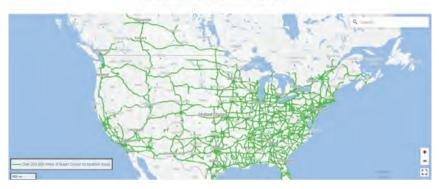
The Super Cruise driver assistance feature uses a LiDAR-scanned map database, which restricts system use to compatible highways.
