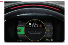
You need to take steering control immediately. A voice prompt will tell you to take over steering control. If you do not take steering control, the vehicle will steer and brake gradually to a stop. Super Cruise will not be available until the next ignition cycle.
