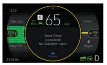
Immediately after Super Cruise disengagement, press the Super Cruise button (within 10 seconds) to display a message with the reason for disengagement.
