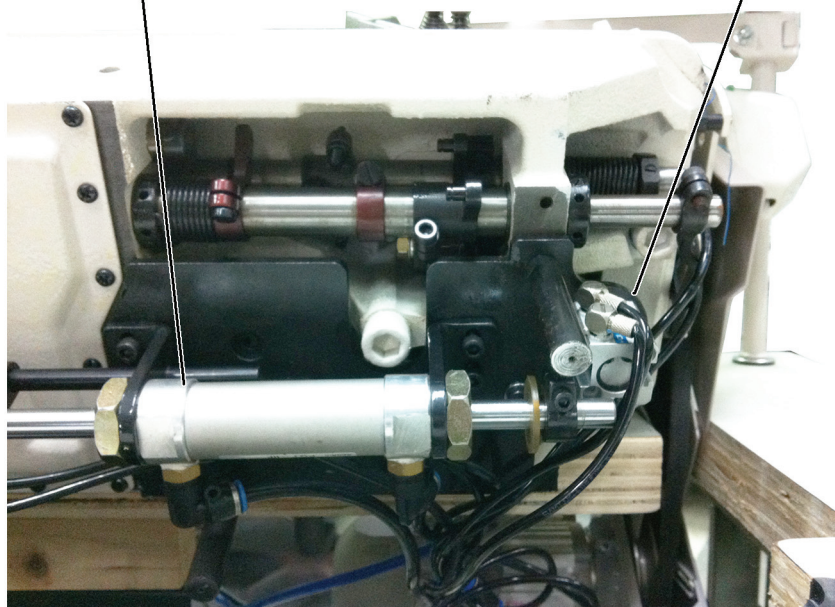
面綫鬆綫氣缸 surface thread release air cylinder
