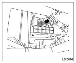
2. Lift upward to release the filter cover and remove the filter cover.
