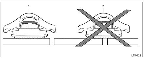
1 correct installation, 2 incorrect installation
