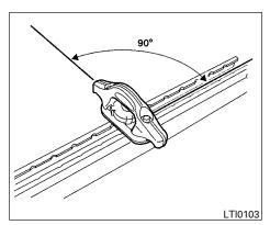
Insert the cleat into the channel perpendicular to the channel as shown. Then rotate the cleat clockwise 90° and slide it to the desired location.
