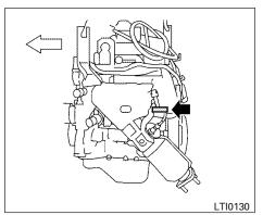
**QR25DE** engine **ENGINE SERIAL NUMBER**
