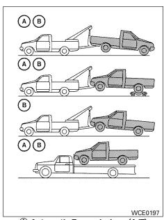
(A) Automatic Transmissions (A/T) (B) Manual Transmissions (M/T) TOWING RECOMMENDED BY NISSAN
