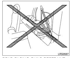
REAR-FACING CHILD RESTRAINT INSTALLATION USING THE SEAT BELTS — PASSENGER'S SIDE JUMP SEAT (King cab models only)
