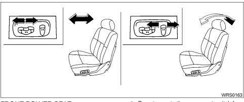
The reclining feature allows adjustment of the seatback for occupants of different sizes for added comfort and to help obtain proper seat belt fit (see "Precautions on seat belt usage" later in this section). Also, the seatback can be reclined to allow occupants to rest when the vehicle is stopped and the transmission is in P (Park) or N (Neutral) position with the parking brake fully applied.
