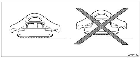
5. There should be no gap between the bottom of the cleat and the top of the channel. Tighten the center bolt hand tight (20-40 inch pounds).
