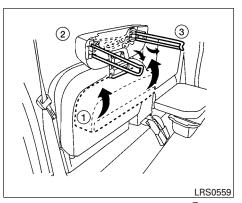
1. To access the jump seat extension (1) on the passenger's side jump seat only pull up (2) on the extension to unfold it to the open position. Then unfold the two support legs 3 and lower the jump seat to the full open 4 seating position.
