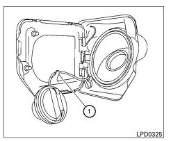
Loop the tether strap around the hook (1) while refuelina.
