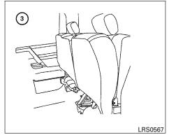
Repeat this process to raise and secure the seat cushion on the other side of the vehicle for maximum storage capacity.
