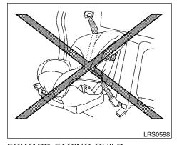
FOWARD-FACING CHILD RESTRAINT INSTALLATION USING THE SEAT BELTS — FRONT PASSENGER AND PASSENGER'S SIDE JUMP SEAT (King cab models only)
