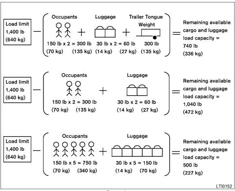
Steps for determining correct load limit
