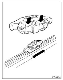
4. Position the cleat so the nubs on the bottom fully seat into the channel detents.
