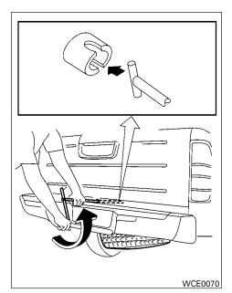
3. Seat the T-shaped end of the jack rod into the T-shaped opening of the spare tire winch. Apply pressure to keep the jack rod engaged in the spare tire winch and turn the jack rod counterclockwise to lower the spare tire.  Once the spare tire is completely lowered, reach under the vehicle, remove the retainer chain, and carefully slide the tire from under the rear of the vehicle.
