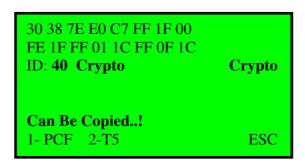
This shows that only the transponder's ID part can be copied, when you see this ,there is no probability to start the car. And the ID 40 transponder, which is in the example, is locked and can not be identified to another car with another device
