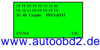
Transpronics, can copy 90% of transponders that are in Volkswagen and Ford cars, it also has detailed data about the transponder. For example, a transponder that has never programmed before has this information below. This transponder's ID part can be copied to a T5 or an ID 33 transponder but cannot start the car.
