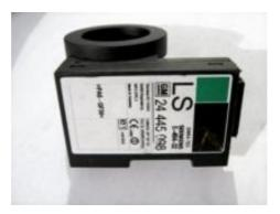
In the immobilizer unite seen above, there is a processor named TMS370C702. After this eeprom is read you have to send it to our machine. (Processor must be read as a \*Bin file)
