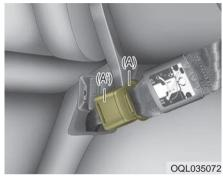
Insert the tongue plate (A) into the buckle (A') until an audible "click" is heard, indicating the latch is locked. Make sure the belt is not twisted.
