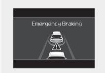
It will operate if the vehicle speed is greater than 8 km/h (5 mph) and less than or equal to 60 km/h (38 mph) on a forward vehicle. (Depending on the condition of the vehicle ahead and the environment surrounding it, the possible maximum operating speed may be reduced.)
