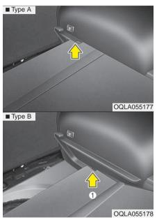
If the vehicle is equipped with a TMK (Tire Mobility Kit) or a temporary tire, you can make the luggage board to flat (Type A) or lower it another level (Type B) for more luggage storage. When you use the luggage board (Type B), you should put it between guides (1).
