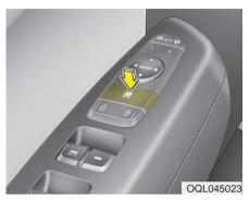
• The driver can disable the power window switches on the rear seat doors by pressing the power window lock button located on the driver's door to the LOCK position (pressed).
