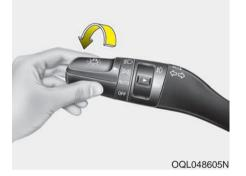
When the light switch is in the parking light position, the tail, license and instrument panel lights will turn ON. Headlight position (ED)
