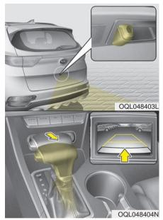
The rear view monitor will activate with the ignition switch ON and the shift lever in the R (Reverse) position.
