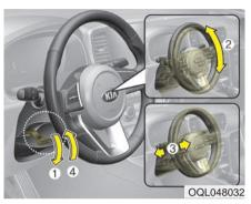
To change the steering wheel angle, pull down the lock-release lever (1), adjust the steering wheel to the desired angle (2) and height (3, if equipped) then pull up the lockrelease lever to lock (4) the steering wheel in place. Be sure to adjust the steering wheel to the desired position before driving.
