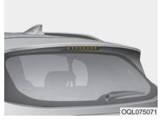
If the high mounted stop lamp (LED type) does not operate, we recommend that you have your vehicle checked by an authorized Kia dealer.
