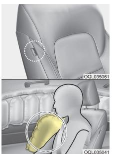
\* The actual air bags in the vehicle may differ from the illustration. Your vehicle is equipped with a side air bag in each front seat. The purpose of the air bag is to provide the vehicle's driver and/or the front passenger with additional protection than that offered by the seat belt alone.
