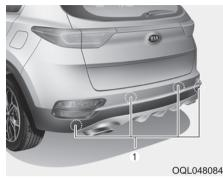
The parking distance warning-reverse assists the driver during backward movement of the vehicle by chiming if any object is sensed within a distance of 120 cm (47 in.) behind the vehicle.
