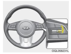
If any method other than the CRUISE ON-OFF switch was used to cancel cruising speed and the system is still activated, the most recent set speed will automatically resume
