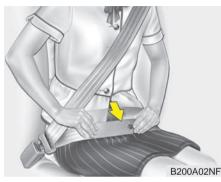
The seat belt automatically adjusts to the proper length only after the lap belt portion is adjusted manually so that it fits snugly around your hips. If you lean forward in a slow, easy motion, the belt will extend and let you move around. If there is a sudden stop or impact, however, the belt will lock into position. It will also lock if you try to lean forward too quickly.
