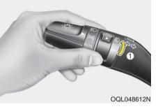
Fog lights are used to provide improved visibility when visibility is poor due to fog, rain or snow, etc. The fog lights will turn on when the fog light switch (1) is turned to the on position after the headlight is turned on.
