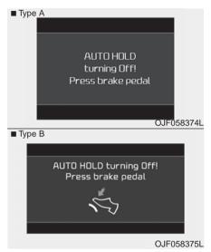
When the conversion from Auto Hold to EPB is not working properly a warning will sound and a message will appear.
