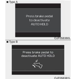
If you do not apply the brake pedal when you release the Auto Hold by pressing the [AUTO HOLD] switch, a warning will sound and a message will appear.
