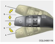
The ignition switch must be on for the turn signals to function. To turn on the turn signals, move the lever up or down (A). The green arrow indicators on the instrument panel indicate which turn signal is operating.
