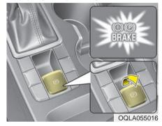
To apply the EPB (electronic parking brake):
