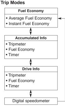
To change the trip mode, scroll the MOVE scroll switch  $(\blacktriangle/ \triangledown)$  in the trip computer mode.
