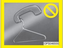
Do not hang other objects such as hangers or hard objects except clothes. Also, do not put heavy, sharp or breakable objects in the pockets of the clothing. In an accident or when the curtain air bag is inflated, it may cause vehicle damage or bodily injury.
