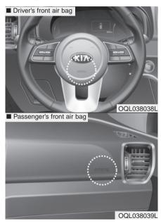
Your vehicle is equipped with an Advanced Supplemental Restraint (Air Bag) System and lap/shoulder belts at both the driver and passenger seating position. The indication of the system's presence are the letters "AIR BAG" located on the air bag pad cover on the steering wheel and the passenger's side front panel pad above the glove box.
