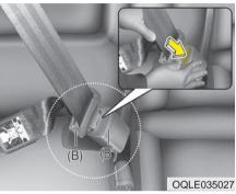
4. Pull the tongue plate (B) and insert it into the buckle (B') until an audible "click" is heard, indicating the latch is locked. Make sure the belt is not twisted.
