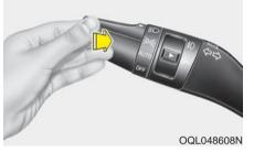
To turn on the high beam headlamp, push the lever away from you. The lever will return to its original position.
