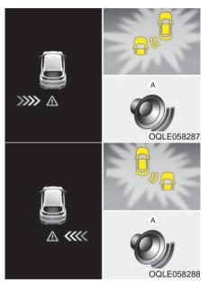
If the vehicle detected by the sensors approaches from the rear left/right side of your vehicle, the warning chime will sound, the warning light on the outside rearview mirror will blink and a message will appear on the LCD display.
