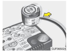
5. Insert the sealant bottle into the housing of the compressor (5) so that the bottle is upright.
