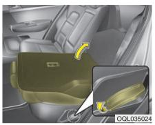
5. To use the rear seat, lift and push the seatback rearward by lifting up the front portion of the folding lever. Push the seatback firmly until it clicks into place. Make sure the seatback is locked in place.
