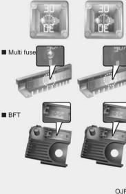
OJF075021 \* Left side : Normal , Right side : Blown A vehicle's electrical system is protected from electrical overload damage by fuses.
