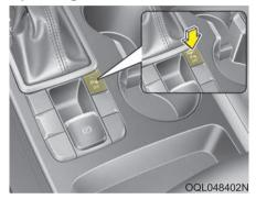
• This system will activate when the indicator on the parking distance warning-reverse OFF button is not illuminated. If you desire to deactivate the parking distance warning-reverse, press the parking distance warning-reverse OFF button again. (The indicator on the button will illuminate.) To turn the system on, press the button again. (The indicator on the button will go off.)
