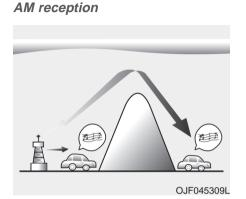
AM broadcasts can be received at greater distances than FM broadcasts. This is because AM radio waves are transmitted at low frequencies. These long distance,low frequency radio waves can follow the curvature of the earth rather than travelling straight. In addition, they curve around obstructions resulting in better signal coverage. FM radio station
