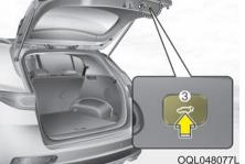
(1) Power liftgate open / close button(2) Power liftgate handle switch
