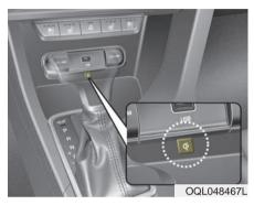
A wireless smart phone charging system located in front of the center console
