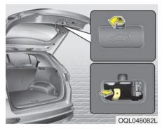
Your vehicle is equipped with an emergency liftgate safety release lever located on the bottom of the liftgate. If someone is inadvertently locked in the cargo area, the liftgate can be opened by pushing the release lever and pushing open the liftgate.
