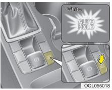
1.Depress the brake pedal, start the engine and then press the Auto Hold button. The white AUTO HOLD indicator will come on indicating the system is in standby.
