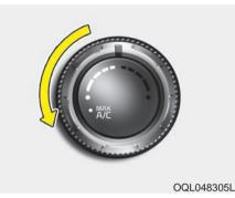
The MAX A/C mode is used to cool the inside of the vehicle faster.
