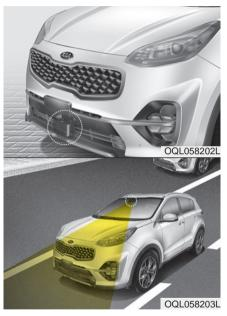
In order for the FCA system to operate properly, always make sure the sensor or sensor cover are clean and free of dirt, snow, and debris. Dirt, snow, or foreign substances on the lens may adversely affect the sensing performance of the sensor.
