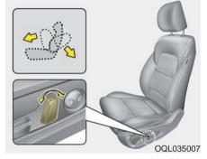
Push the control switch forward or backward to move the seatback to the desired angle. Release the switch once the seat reaches the desired position. Seat height
