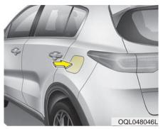
1. To open the fuel filler lid, press the 3 o`clock position edge of the fuel filler lid.
