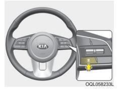
When the Smart Cruise Control System is ON, you can set and maintain the distance to the vehicle ahead without pressing the accelerator or brake pedal.
