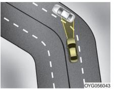
Your vehicle speed can be reduced due to a vehicle in the adjacent lane. Adjust your speed by depressing the brake pedal or applying the accelerator pedal according to road and driving conditions ahead. Check to be sure that the road conditions permit safe operation of the smart cruise control.
