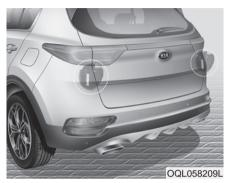
The sensors are located inside the rear bumper for detecting rear/side areas.
