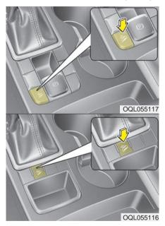
The Downhill Brake Control (DBC) allows the vehicle to descend from a steep hill without depressing the brake pedal. It slows down the vehicle under 8 km/h (5 mph) and allows the driver concentrate on steering the vehicle.
