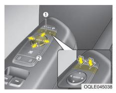
The electric remote control mirror switch allows you to adjust the position of the left and right outside rearview mirrors. To adjust the position of either mirror, press the R or L button (1) to select the right side mirror or the left side mirror, then press a corresponding point ( $\blacktriangle$ ) on the mirror adjustment control to position the selected mirror up, down, left or right.
