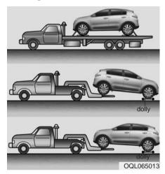
If emergency towing is necessary, we recommend having it done by an authorized Kia dealer or a commercial tow-truck service. Proper lifting and towing procedures are necessary to prevent damage to the vehicle. The use of wheel dollies or flatbed is recommended. On AWD vehicles, your vehicle must be towed with a wheel lift and dollies or flatbed equipment with all the wheels off the ground.
