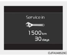
When Service Required is set, the remaining distance/time before service is required appears on the LCD screen.
