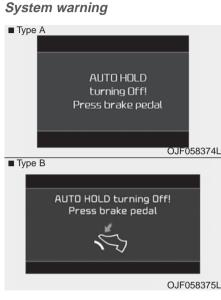
When the conversion from Auto Hold to EPB is not working properly a warning will sound and a message will appear.
