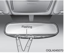
When programming the buttons for the first time, press and hold the left and center buttons (⊕, ①) simultaneously until the indicator light begins to flash after approximately 20 seconds. (This procedure erases the factory-set default codes. Do not perform this step when programming the additional HomeLink buttons.)
