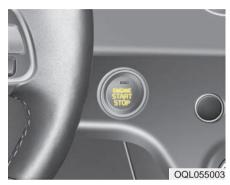
Whenever the front door is opened, the ENGINE START/STOP button will illuminate for your convenience. The light will go off after about 30 seconds when the door is closed.
