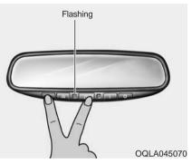
To erase the three programmed buttons (individual buttons cannot be erased):
