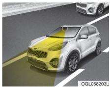
In order for the FCA system to operate properly, always make sure the sensor are clean and free of dirt, snow, and debris.
