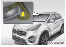
The Lane Keeping Assist (LKA) system is designed to detect the lane markers on the road with a front view camera at the front windshield, and assists the driver's steering to help keep the vehicle in the lanes. When the system detects the vehicle straying from its lane, it alerts the driver with a visual and audible warning, while applying a slight countersteering torque, trying to prevent the vehicle from moving out of its lane.
