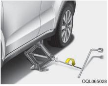
8. Insert the wheel lug nut wrench into the jack and turn it clockwise, raising the vehicle until the tire just clears the ground. This measurement is approximately 30 mm (1 in.).
