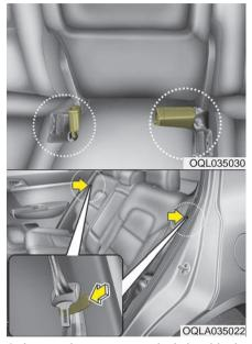
3. Insert the rear seat belt buckle in the pocket between the rear seatback and cushion, and insert the rear seat belt webbing in the guide to prevent the seat belt from being damaged.
