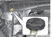
2. Make sure that the tiny protrusions inside the coolant cap are securely interlocked.
