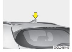
The shark fin antenna will receive the AM, FM broadcast signals and transmit data.
