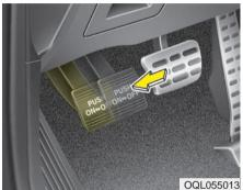
To engage the parking brake, first apply the foot brake and then depress the parking brake pedal down as far as possible.
