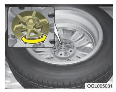
Turn the tire hold-down wing bolt counterclockwise.
