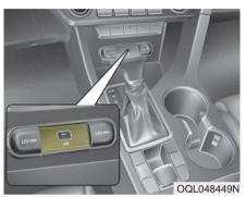
You can use the USB port to plug in a USB device or iPod<sup>®</sup>.
