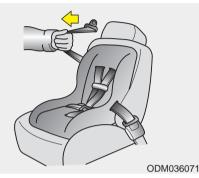
3. Pull the shoulder portion of the seat belt all the way out. When the shoulder portion of the seat belt is fully extended, it will shift the retractor to the "Automatic Locking" (child restraint) mode.
