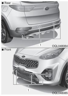
The parking distance warning assists the driver during movement of the vehicle by chiming if any object is sensed within the distance of 100 cm (39 in.) in front and 120 cm (47 in.) behind the vehicle. This system is a supplemental system and it is not intended to nor does it replace the need for extreme care and attention of the driver.
