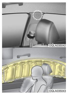
\* The actual air bags in the vehicle may differ from the illustration. Curtain air bags are located along both sides of the roof rails above the front and rear doors.
