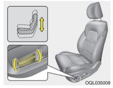
Pull the front portion of the control switch up to raise or press down to lower the front part of the seat cushion. Pull the rear portion of the control switch up to raise or press down to lower the seat cushion. Release the switch once the seat reaches the desired position.
