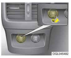
The USB charger is designed to recharge batteries of small size electrical devices using a USB cable. The electrical devices can be recharged when the Engine Start/Stop button is in ACC/ON/START position.
