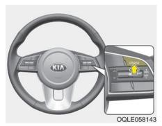
When the Smart Cruise Control System is not needed, press the [CRUISE] switch and deactivate the system.
