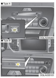
Your vehicle is equipped with an occupant detection system in the front passenger's seat.
