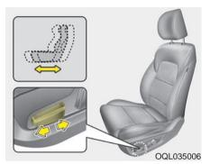
Push the control switch forward or backward to move the seat to the desired position. Release the switch once the seat reaches the desired position. Seatback angle
