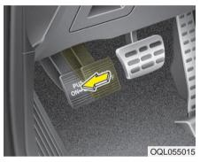
To release the parking brake, depress the parking brake pedal a second time while applying the foot brake. The pedal will automatically extend to the fully released position.
