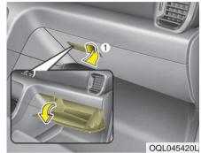
To open the glove box, pull the lever (1) and the glove box will automatically open. Close the glove box after use.
