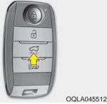
Press the power liftgate close button for approximately one second when the liftgate is opened. The liftgate will close and lock automatically.
