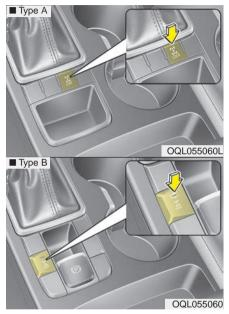
The All Wheel Drive (AWD) system delivers engine power to the front and rear wheels for maximum traction. AWD is useful when extra traction is required on road, such as, when driving on slippery, muddy such as wet, or snow-covered roads. These vehicles are not designed for challenging off-road use.
