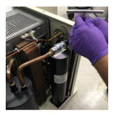
Figure 14 Install Adsorber
