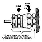
Figure 7 Connect Gas Line to Compressor or Cold Head
