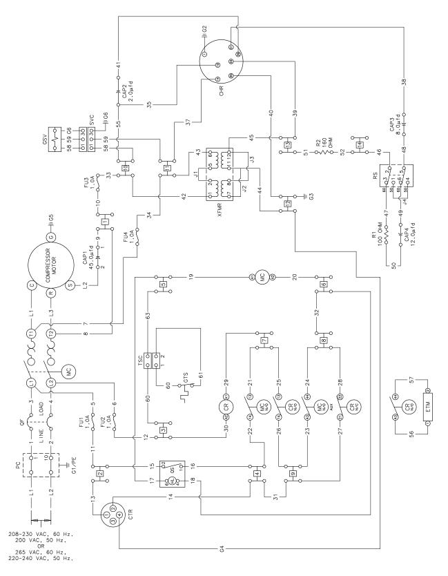
Figure 20 F-20L Compressor Wiring Schematic
