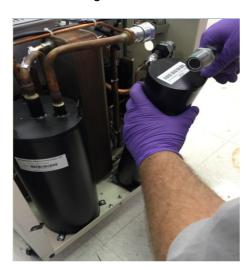
Figure 12 Remove Adsorber
