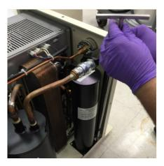
Figure 10 Disconnect Adsorber from Base
