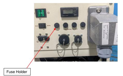
Figure 18 Fuse Holders on F-20L Front Panel
