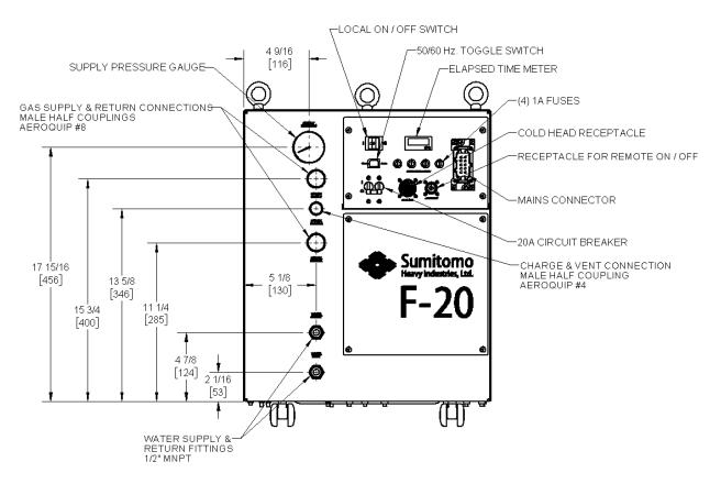
Figure 2 F-20L Compressor, Front View
