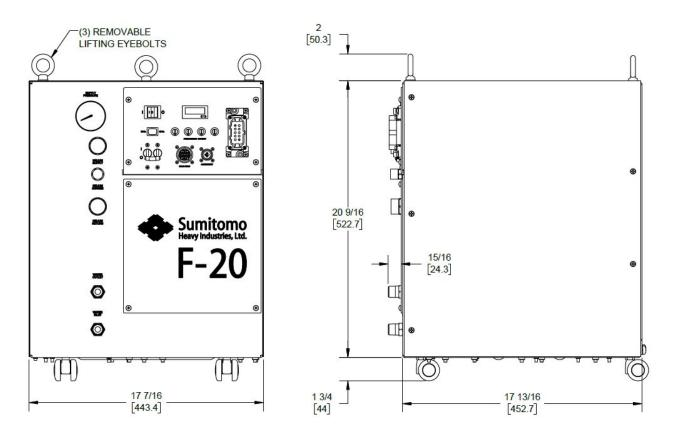
Figure 3 F-20L Compressor, Dimensions
