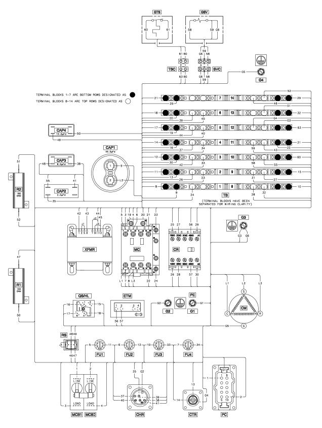
Figure 19 F-20L Compressor Wiring Diagram
