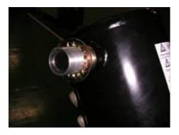
Figure 13 Install Lock Washer on Adsorber
