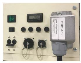
Figure 4 Connect Mains Power Supply Cable to Mains Power Receptacle
