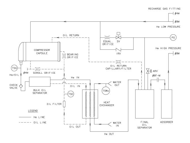
Figure 1 Compressor Flow Diagram
