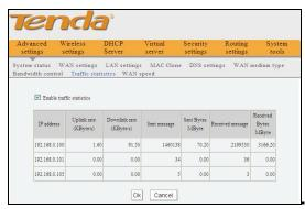
**Enable Traffic statistics**: It is used to calculate the traffic used by the LAN computers. You can enable it to calculate the traffic for you. Usually, disable it to improve the router's data packet processing ability, and the default is disabled. When this function is enabled, the webpage will refresh automatically every five minutes, meanwhile, each computer's traffic value will refresh automatically.
