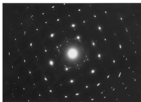
b: Selected area diffraction image
