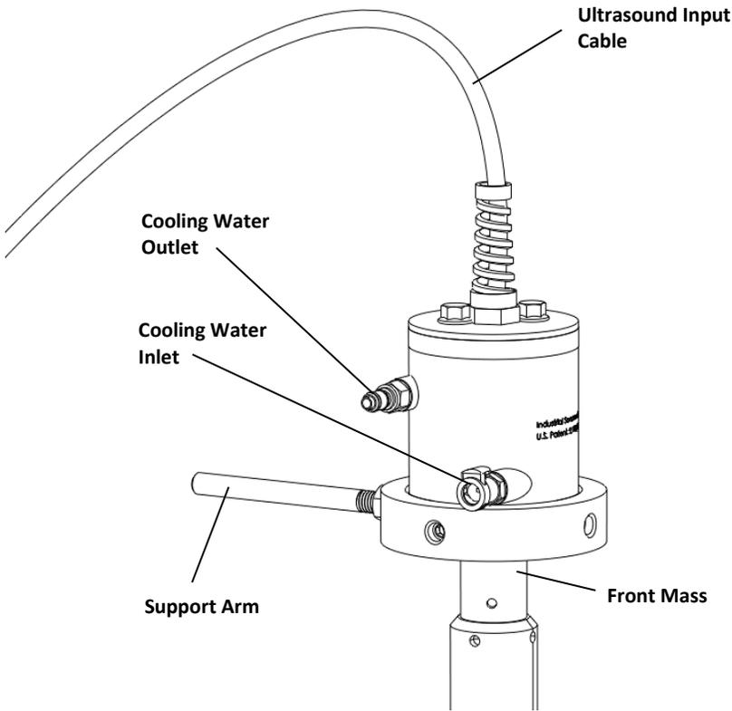
Figure 10. SWCT-3600 ultrasonic transducer.
