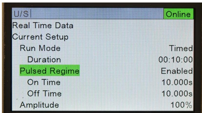
7. To adjust the amplitude, press **AMP**, then use the **+/-**, **←/→** and **ENTER** keys to change and set the amplitude:
