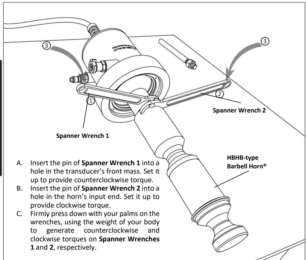
**Figure 12.** Attaching a Barbell Horn® to the SWCT-1200 transducer.
