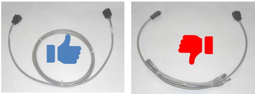
**Figure 6.** Proper cable slack take-up.
