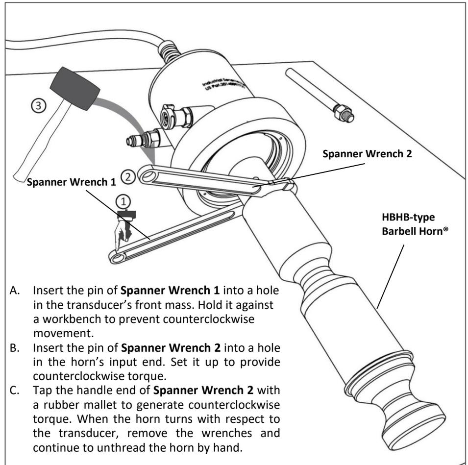
**Figure 13.** Removing a Barbell Horn® from the SWCT-1200 transducer.
