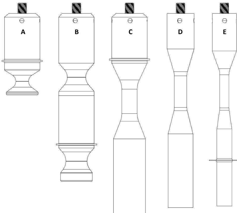
**Figure 11.** Barbell Horns® compatible with the ISP-3600 ultrasonic processor. A – HBH-F20D45G4.1s; B – HBHB-F20D45G5s; C – FBH-F20D47G3.5s; D – FBH-F20D35G3.8s; E – FBH-F20D21G5s.
