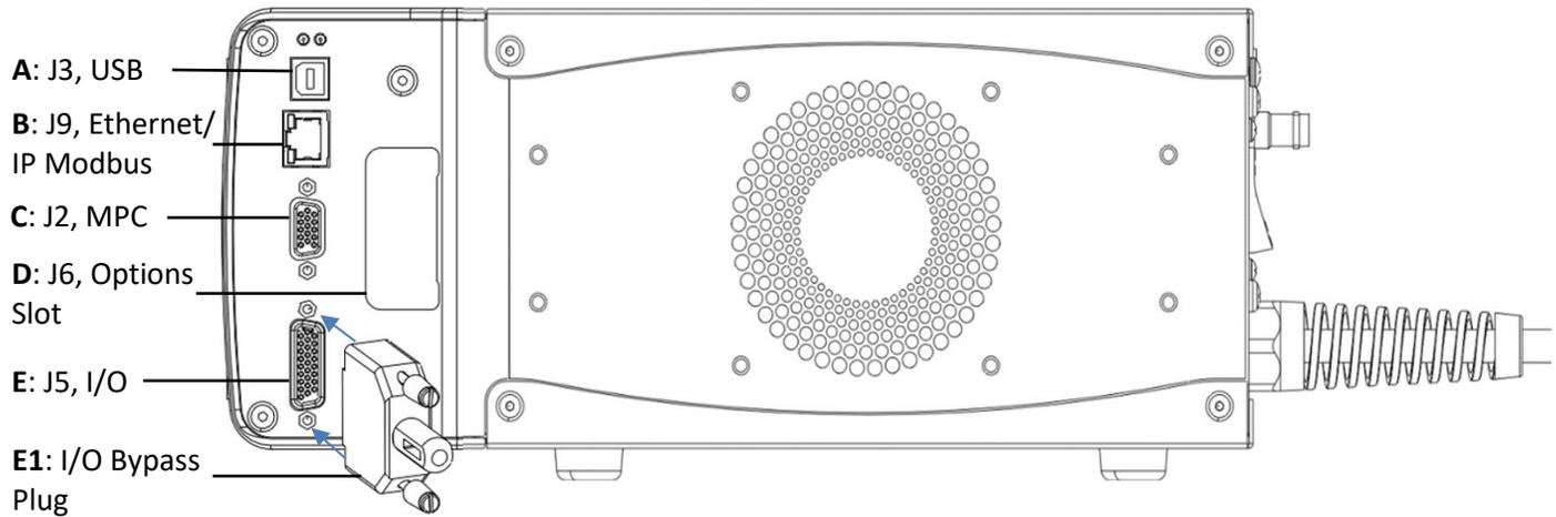
**Figure 4.** Side view of the generator.
