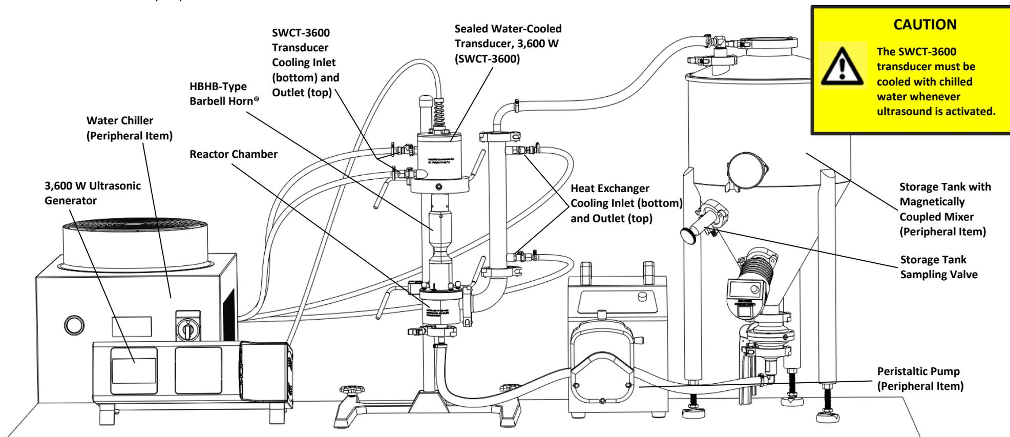
**Figure 2.** ISP-3600 ultrasonic processor configured in the recirculating flow-through mode. The 3,600 W ultrasonic generator excites vibration in the SWCT-3600 transducer. The vibration amplitude is amplified by the HBHB-type Barbell Horn®, and the ultrasonic energy is delivered to the processed liquid flowing through the reactor chamber. Typical liquid volumes processed with this setup are 10 – 1000 L. Much large volumes can be processed as well, with no upper limit.
