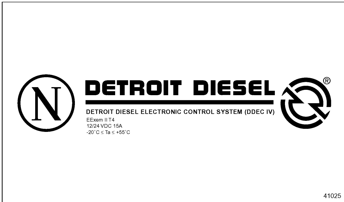
Figure 8-15 Group II Zone 2 (Category 3) Top of the Cylinder Head with Vinyl Rocker Cover Label — Series 60
