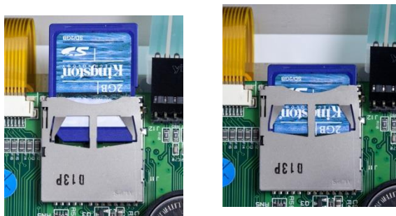
Figure 1-6: Sliding an SD Card into the SD Socket (left); SD Card Installed (right)
