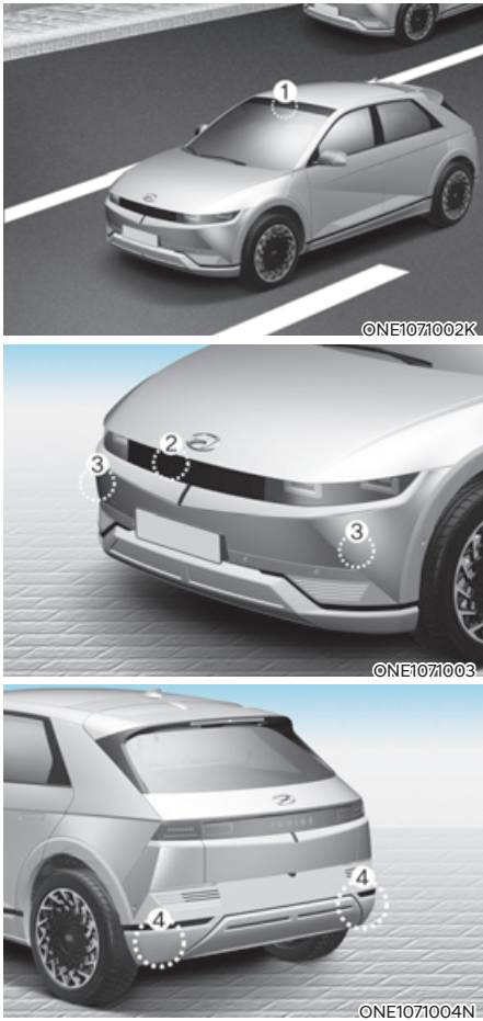
[1] : Front view camera, [2]: Front radar, [3] : Front corner radar (if equipped), [4] : Rear corner radar (if equipped)
