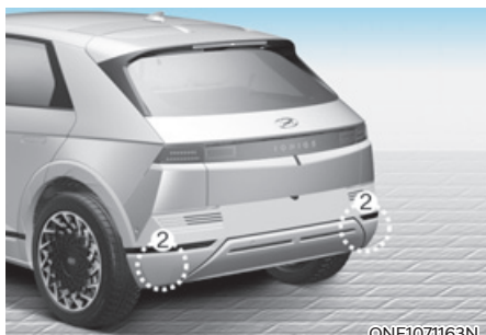
[1] : Front view camera, [2] : Rear corner radar
