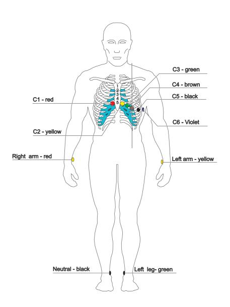
A minimal resistance between skin and electrode is required to obtain the best ECG signal and ensure the highest quality ECG recording. Therefore please note the follo-
