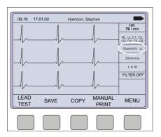
To reduce the possibility of overlapping traces, an auto sensitivity reduction is applied in Auto Mode (default). This means that the unit detects very large waveform amplitudes and sets the sensitivity for the extremity and/or precordial leads to 5 mm/mV. An 'A' by the side of the sensitivity indicates that Auto sensitivity is set. To disable this function, the AUTO SENSITIVITY key (key 3) must be pressed.
