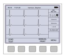
If an electrode resistance is too high for a good recording, or an electrode becomes dislodged during a recording, the electrode indication (1) flashes on the screen and an audible beep is heard. The electrode(s) must be reapplied.
