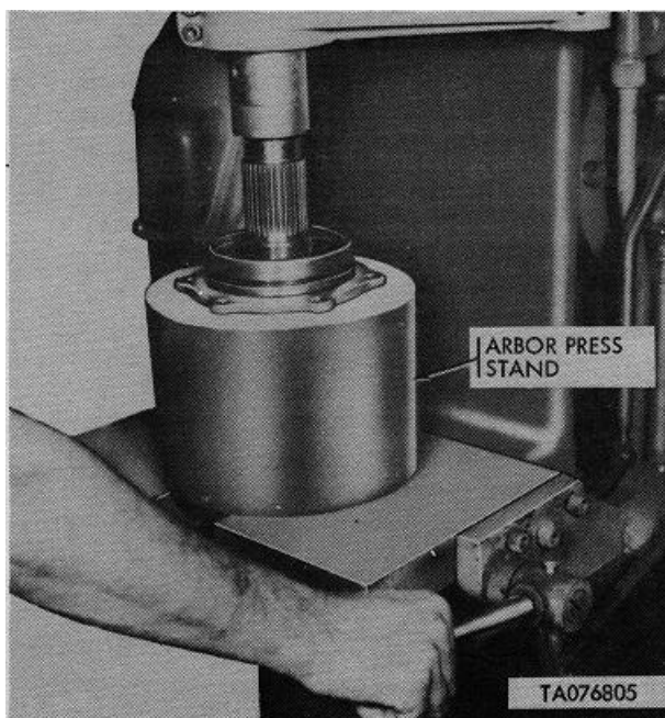
Figure 4-28. Output Shaft Removal from Bearing Cap Using Arbor Press Stand
