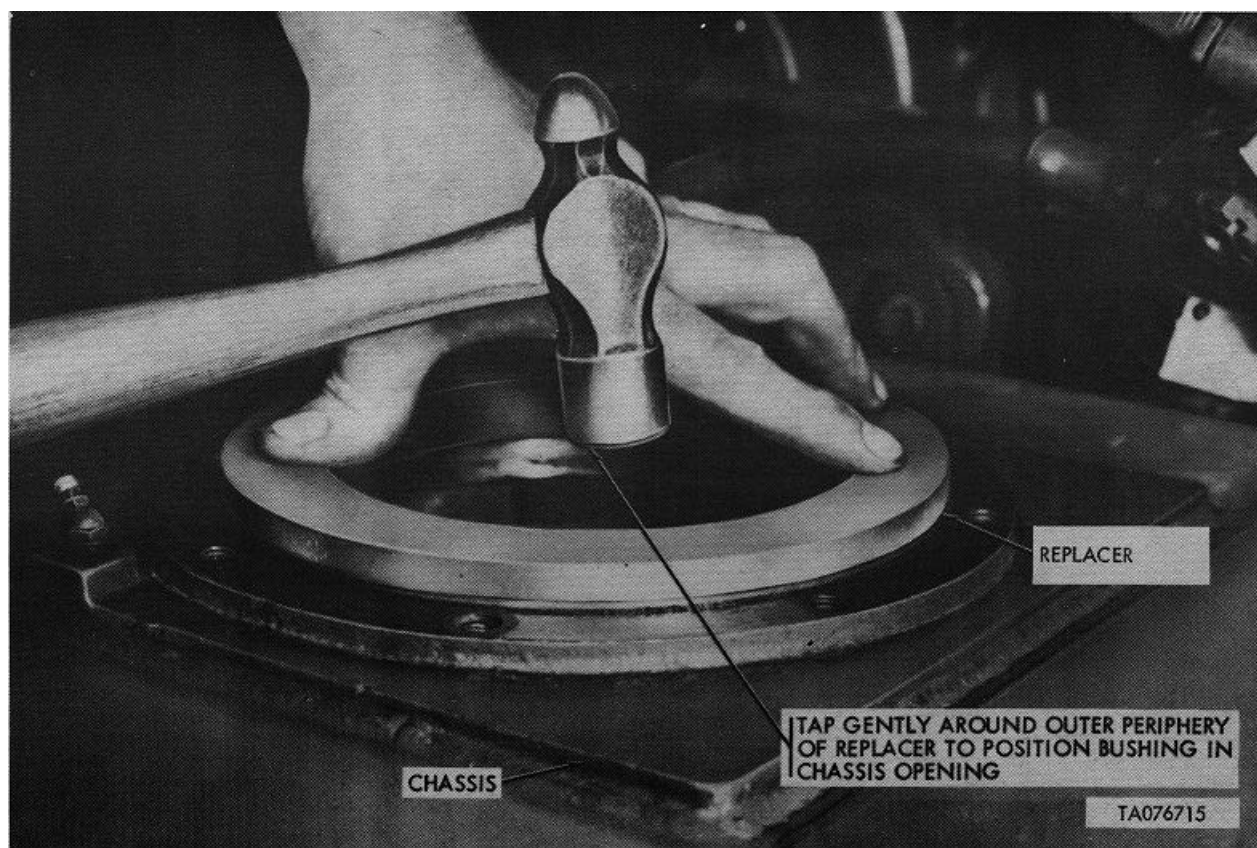
Figure 3-23. Main Support - Bushing Installation Using Replacer
