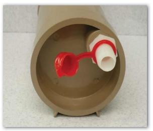
The photograph at the left shows the inflow side of the DD2011. Note that the inflow port is "off axis". This side of the separator is connected to the HVE line coming from the patient. Note the red vinyl cover over the 5/8 inch inflow port of the separator. When the separator is loaded with debris and needs changing, the red vinyl cover is placed over the port to prevent any leakage of debris from the separator.
