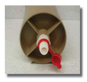
The photograph at the left shows the outflow side of the DD2011. Note that the outflow port is in line with the long axis of the separator. This side of the separator is connected to the vacuum source. Note the red vinyl cover over the 5/8 inch outflow port of the separator. When the separator is loaded with debris and needs changing, the red vinyl cover is placed over the port to prevent any leakage of debris from the separator.
