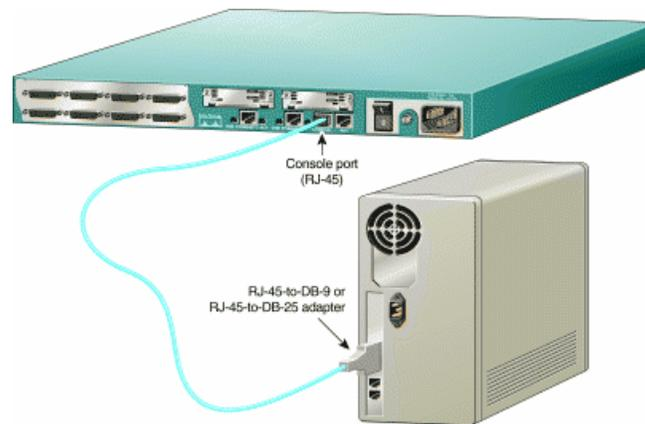
**Figure 1.3** Connection of Console Cable
