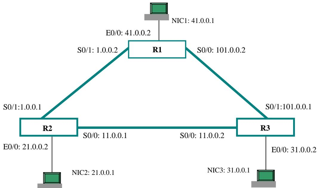
**Figure 2.1** Interconnection of the devices
