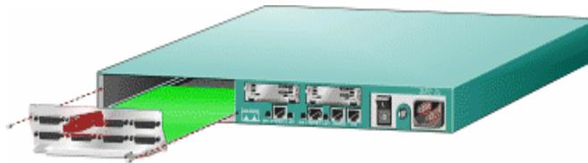
**Figure 1.2** Cisco 2600 Router Rear View
