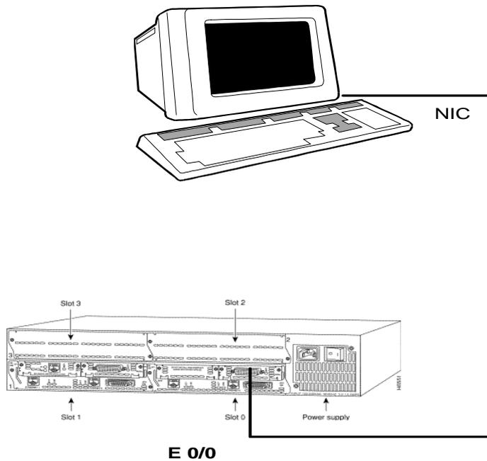
**Figure 1.5** Connection of PC's NIC to router
