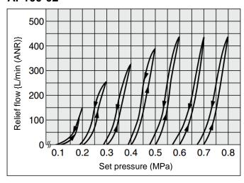
Note) The graph above shows the relief flow when the set pressure rises and falls from 0.1MPa.
